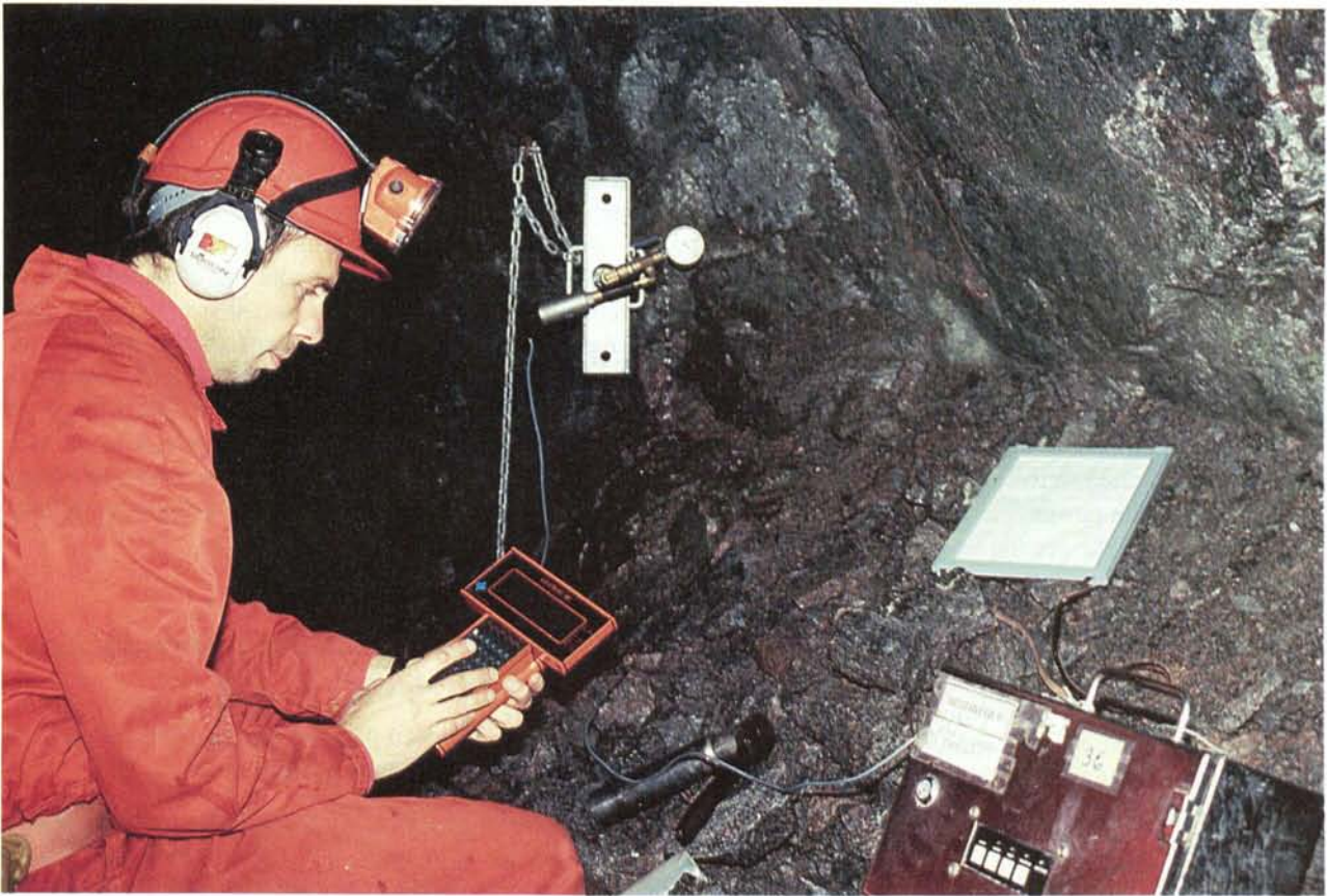
Figure 12-5. After every fourth "round", two 20 m long investigation holes are drilled in front of the tunnel. The hydraulic injection test is performed to measure water permeability (transmissivity).
