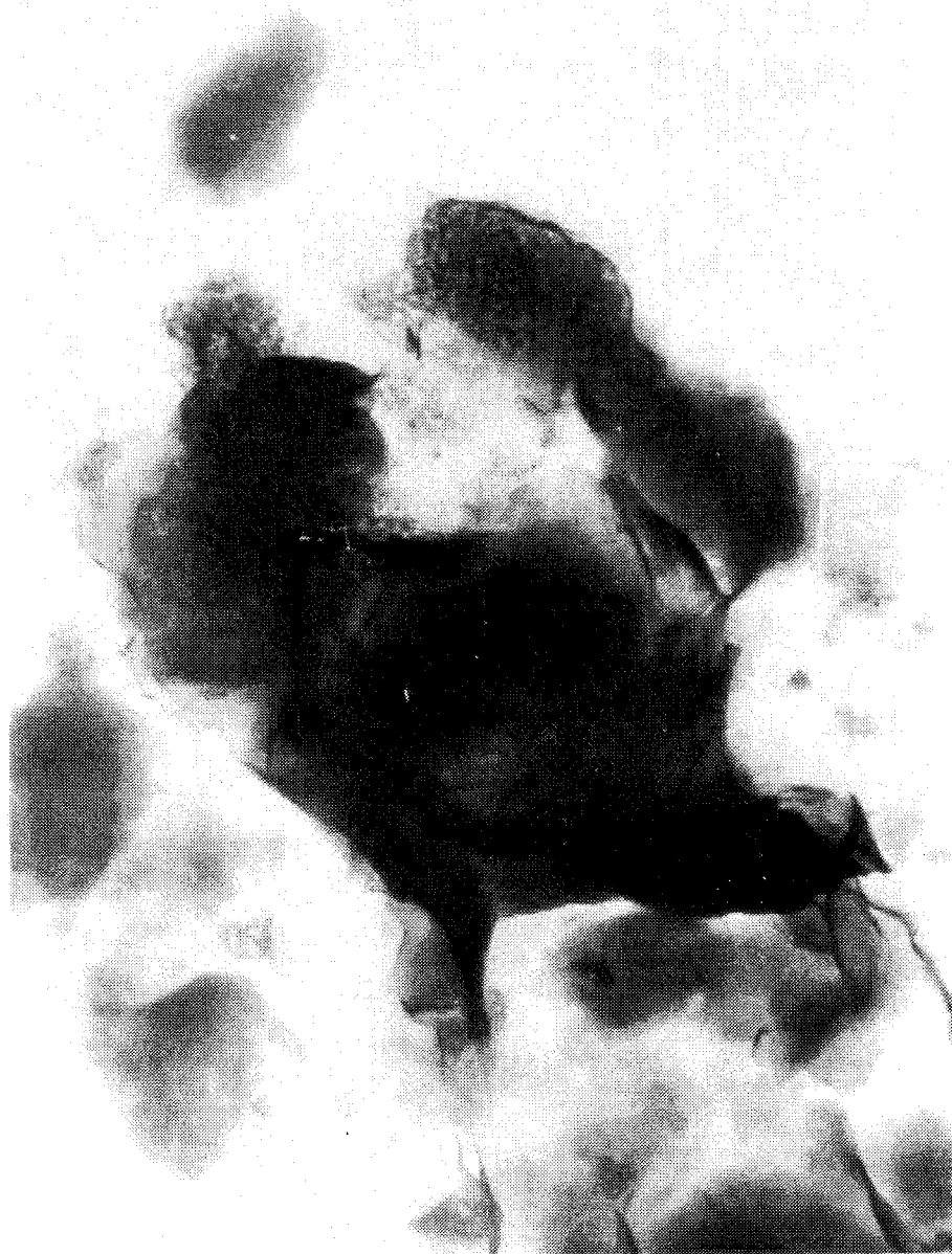
Figure 30 TEM Micrograph of metal tube sample N-024-B washed 4x with 0.05 M HEPES Buffer. Few bacteria and difficult to find.
