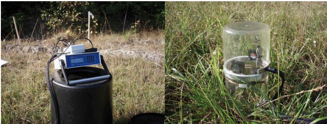
Figure 3-1. EGM-4 gas monitor for CO 2 to the left, and CPY-2 chamber for closed systems to the right. Both instruments from PP Systems.
