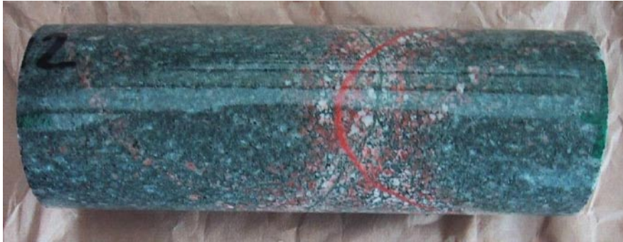
Figure 5-3. Sample KFM05A 692.00 m. Sealed fracture with hematite stained adularia cutting an older epidote sealed fracture. The diameter of the drill core is ~ 5 cm.
