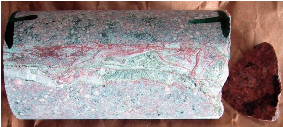
Figure 5-1. KFM05A 395.75 m. Fracture sealed with hematite stained adularia (red), prehnite (greenish) and calcite (white). The diameter of the drill core is c. 5 cm.
