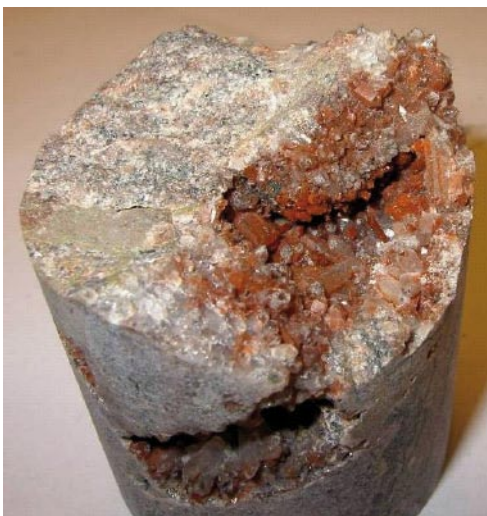
Figure 5-6. Sample KFM07A 876.11 m. Euhedral quartz and adularia crystals in a large void in the rock. The reddish colour is due to sub-microscopic grains of hematite. The diameter of the drill core is ~ 5 cm.
