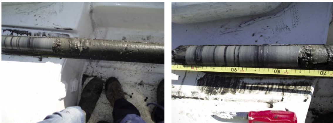
Figure 5-2. Sediments from Kallrigafjärden. The transition from gyttja to clay (left). To the right is a close-up of the laminated clay. Also seen are the layers with sandy gyttja and sandy gravel with gyttja.
