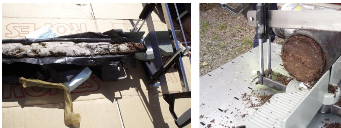
Figure 4-2. Slicing the peat core at Forsmark (left) and at Oskarshamn (right).
