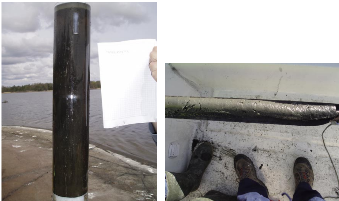
Figure 4-1. Sediment cores sampled with the HTH corer (left) and the russian corer (right).
