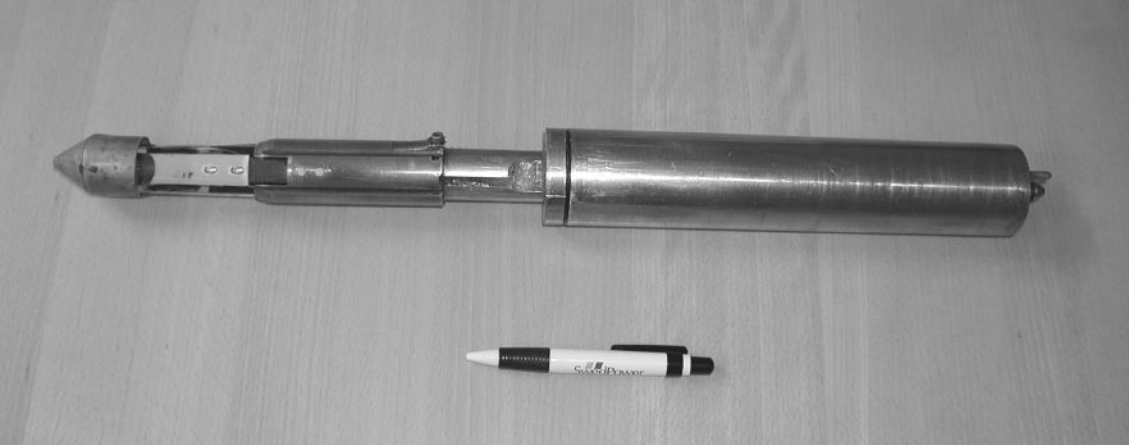
Figure 3-1. The Borre probe.
