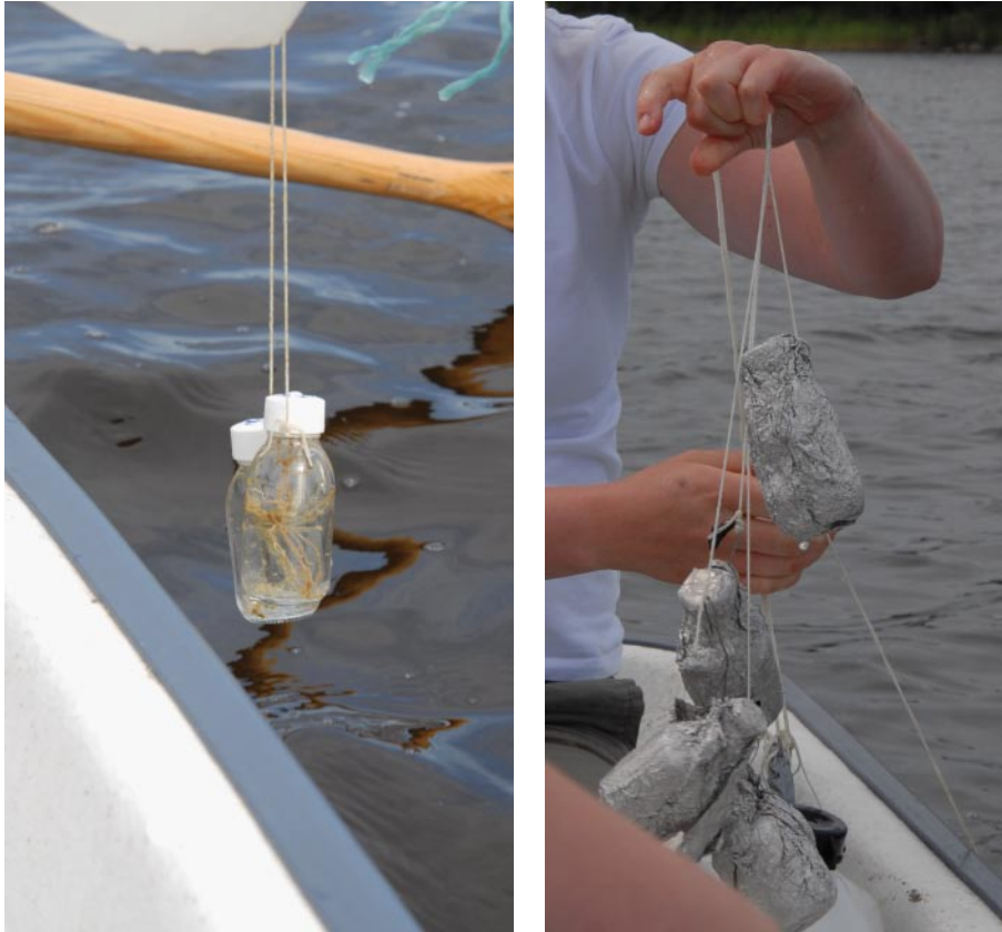
Figure 4-1. Bottles for measurement of primary production (left) and respiration (right).
