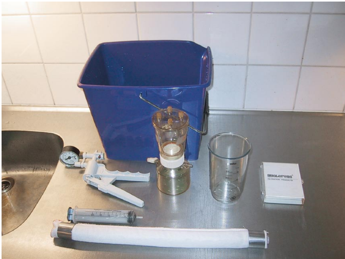
Figure A12-1. The setup for the experiment – the colloid reactor (in the fore front) the vacuum pump, filter holder, filters and a bucket.
