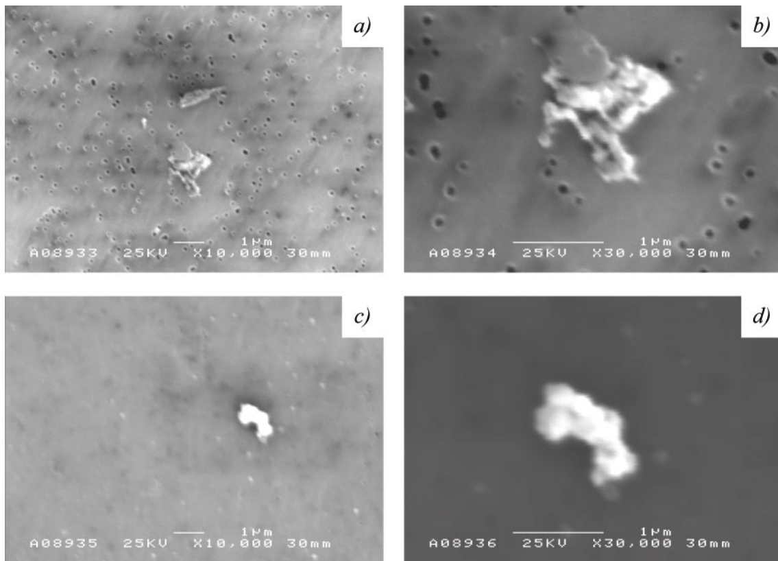
Figure A15-6. PVA1 SEM micrographs of membranes: a) and b) of 0.1 \mu\text{m} membrane magnifications \times 10,000 and \times 30,000 , respectively (prefiltration with a 0.2 \mu\text{m} membrane); c) and d) of 0.05 \mu\text{m} membrane magnifications \times 10,000 and \times 30,000 , respectively (prefiltration with a 0.1 \mu\text{m} membrane).
