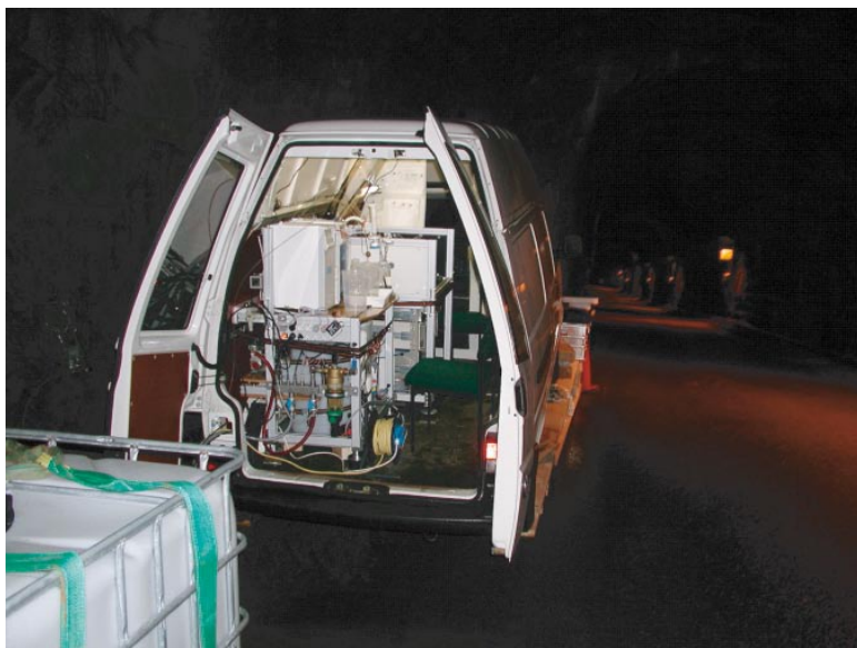
Figure A3-6. LIBD instrumentation in the Äspö Hard Rock Laboratory access tunnel.
