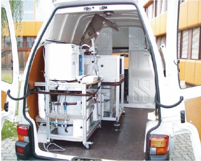
Figure 2-4. The equipment for Laser-Induced Breakdown-Detection (LIBD) of colloids is installed in a van in order to allow mobility and on-line measurements at boreholes /Hauser et al. 2002/.
