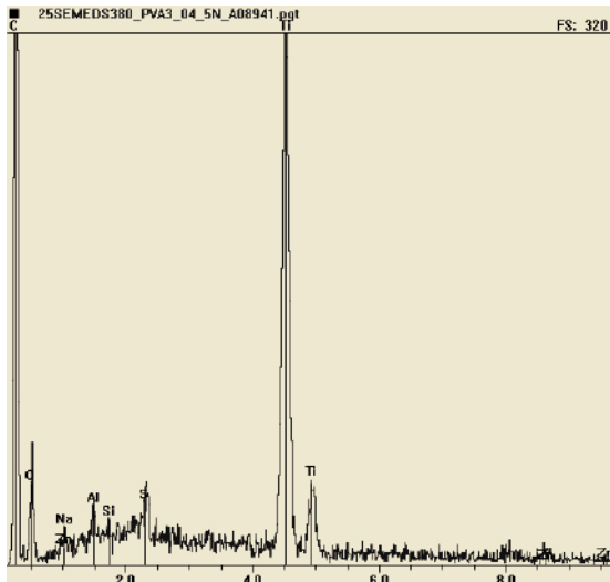
Figure A15-17. EDS spectrum of the above 0.05 \mu\text{m} membrane. Titanium is the main element present, minor amounts of Na, Mg, Al, S and Cl.
