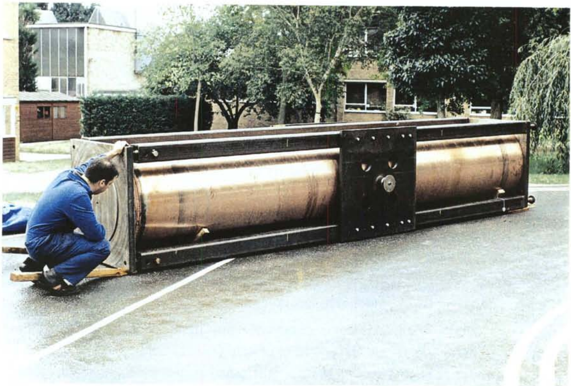
Figure 5.3-1. The canister's copper shell.
