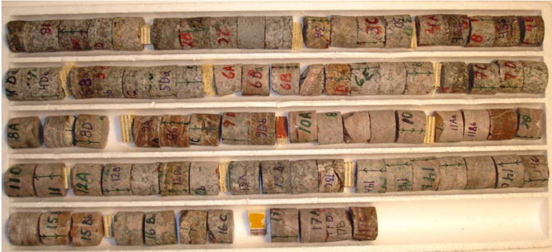
Figure 5-3. Photo of the samples collected across the NE-1 deformation zone (sample KA1240A03 = 8B is missing).
