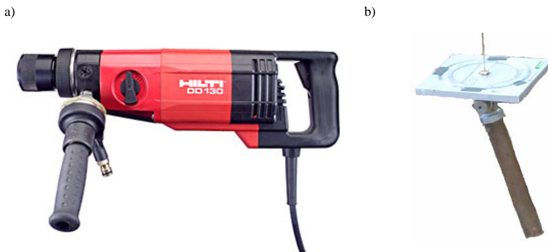
Figure 3-1. a) Drill machine used for the collection of samples. b) Sun compass that measures strike and dip of the drill cores (supplemented by magnetic compass if no sun).
