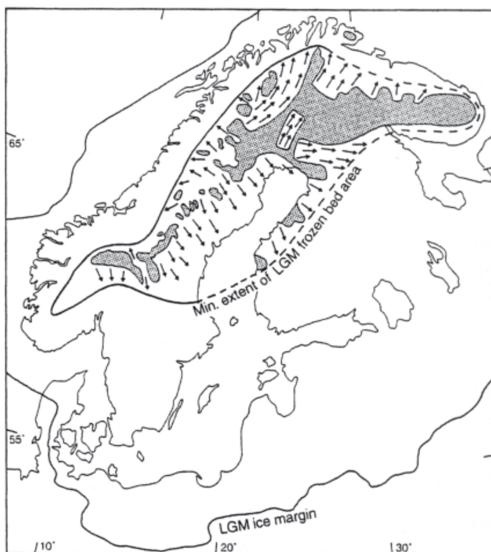
Figure 3-1. Distribution of areas with frozen bed during the deglaciation (shaded areas). The interpreted minimum distribution of frozen bed during LGM is also shown on the map /from Kleman et al. 1997/.
