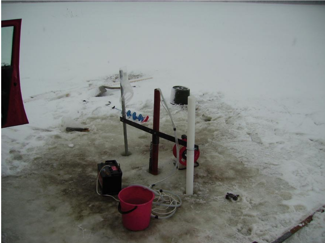
Figure 4-2. Groundwater monitoring well SFM0081 (middle), BAT filter tip SFM0082 for pore pressure measurements (left) and BAT filter tip SFM0083 for water sampling (right), installed below open water in Bolundsfjärden. The BAT casings are anchored with fittings to the groundwater monitoring well. After installation, the groundwater monitoring well was pumped until stable readings of the temperature and the electric conductivity were obtained.
