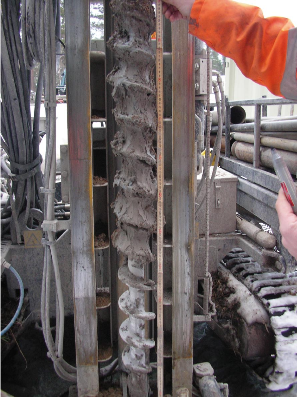
Figure 4-1. Soil sampling by auger drilling in borehole SFM0107.
