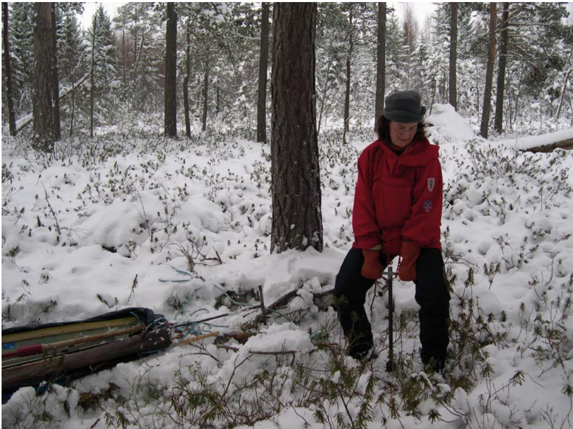
Figure 4-1. Coring with a Russian peat corer in the bog at Wetland 3.
