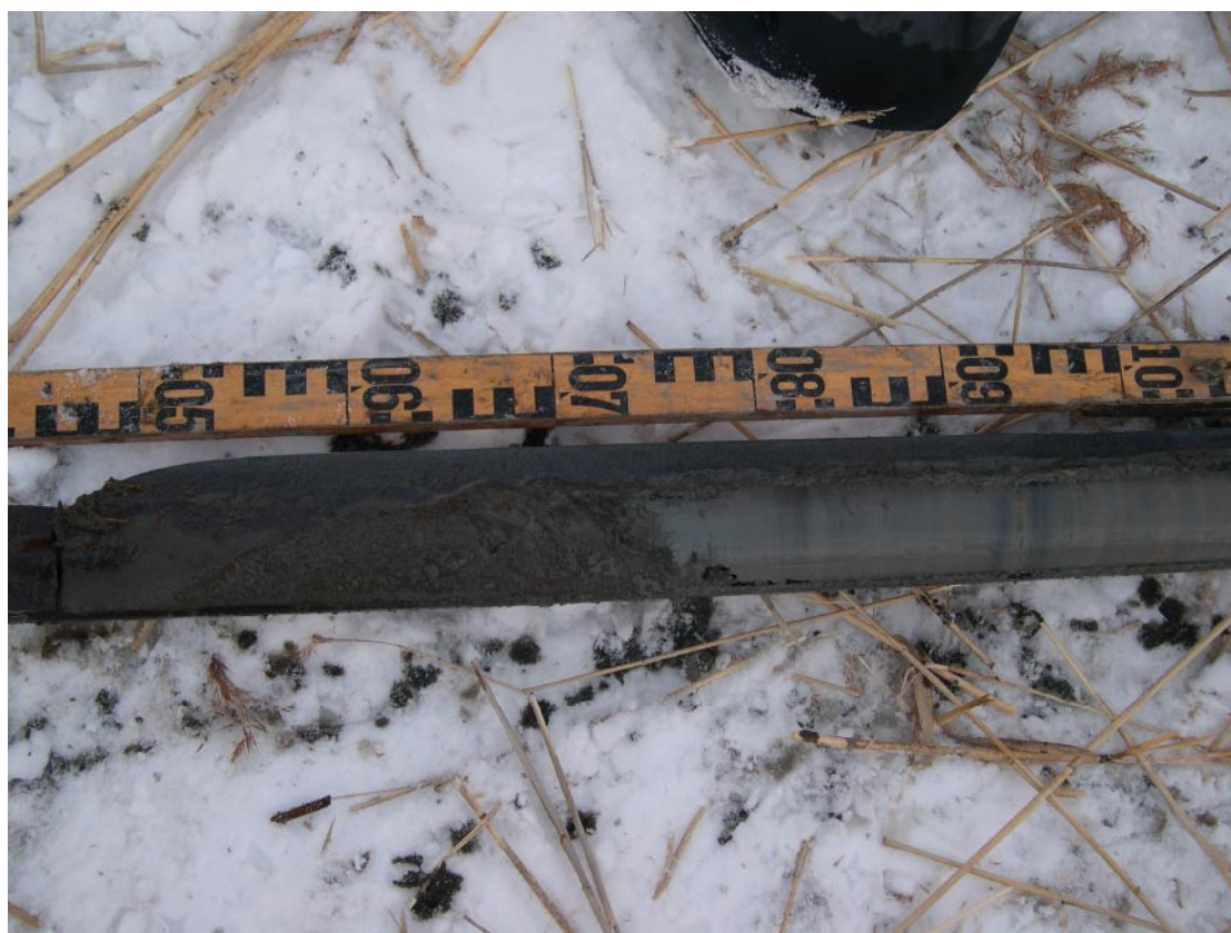
Figure 5-2. Section of core (1.5–2.0 m depth) at SFM0084 showing how the sand is erosively cut into the underlying clay.
