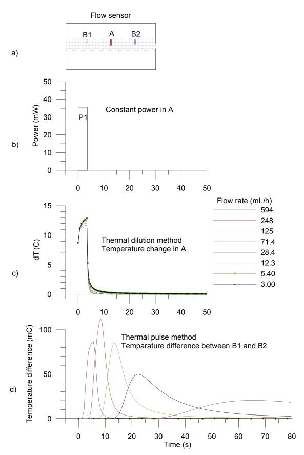
Figure 3-3. Flow measurement, flow rate < 600 mL/h.
