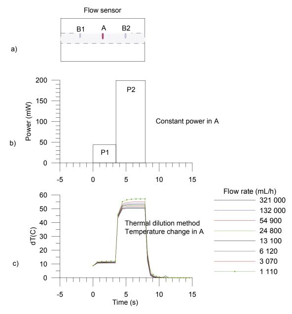
Figure 3-4. Flow measurement, flow rate > 600 mL/h.
