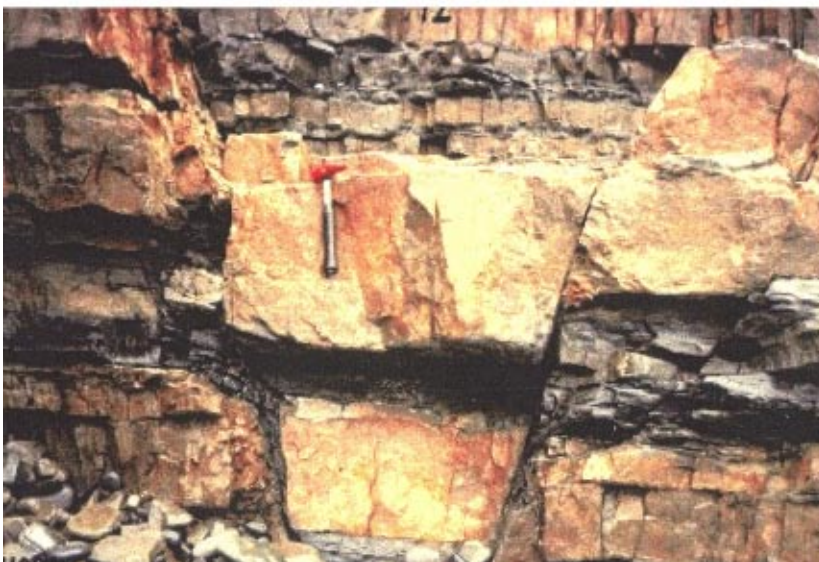
Figure 2-20. Examples of brittle shear failure in which the failure planes become increasingly more and more discrete. Top, shows “granulation seams” in a porous sandstone, Middle more localized shear planes. Bottom, the shear failure is defined by a single fracture plane.
