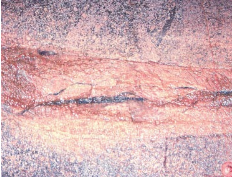
Figure 2-57. An example from the Äspö Hard Rock Laboratory where the movement of fluids through a fracture has precipitated minerals within the fracture, has caused alteration of the wall rock but has not completely sealed the fracture so that it is still significantly conductive.
