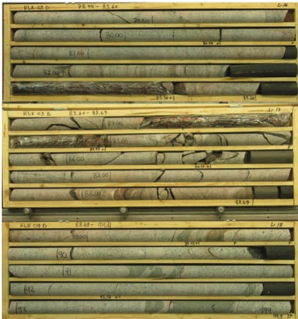
Figure 4-8. Cores from borehole KLX09D for the interval 78.74–94.11 m. The most intensively fractured part of the supposed MDZ occurs at c 82.50–85.0 m.
