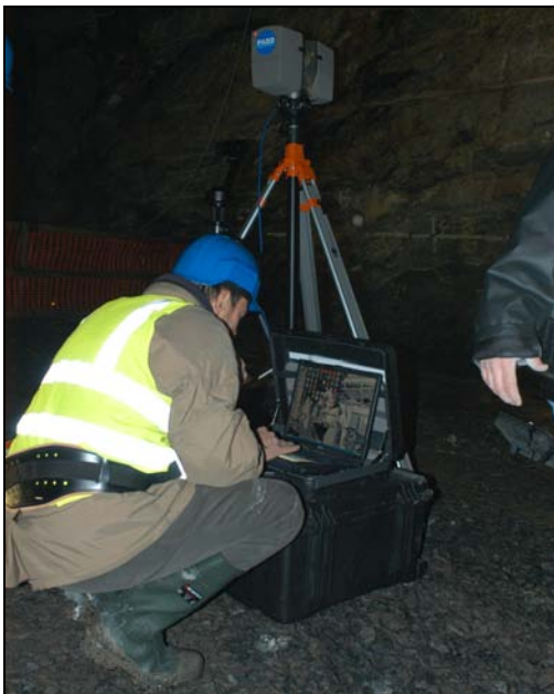
Laser scanning. The laser scanner is on the tripod and the computer that collects the scanning data is on the box on the floor.
