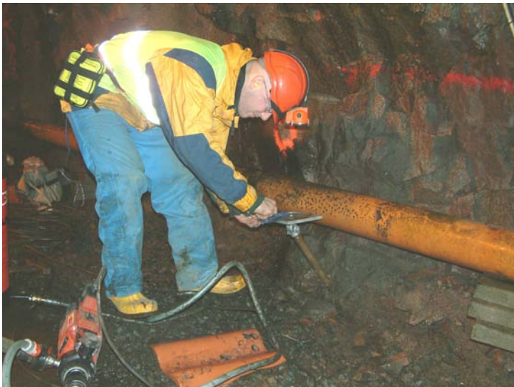
Orientation of drill core by use of magnetic compass, test in the A-tunnel (TASA) of Äspö HRL.
