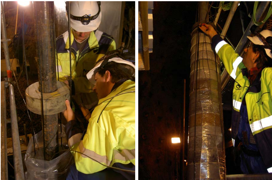
Figure 5-1 Preparation of a test parcel with blocks of alternative buffer materials.
