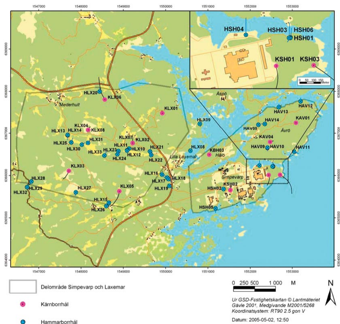
Figure 2-13. Groundwater sampling locations in the Simpevarp area. Location of hydrogeochemically prioritised boreholes KLX01, KLX02, KLX03, KLX04, KLX05, KLX06, KLX07 and KLX08 in the Laxemar subarea. Also indicated are the percussion boreholes (HLX01-33), many of which are included in the Laxemar v.2.1 evaluation.
