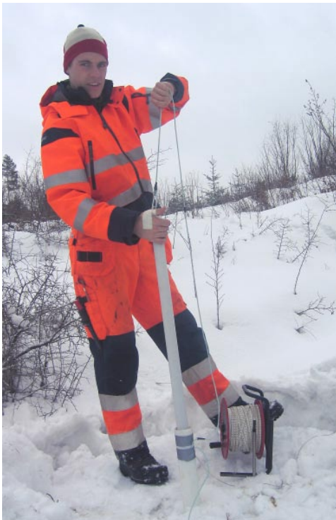
Figure 3-1. Slug and water level meter.
