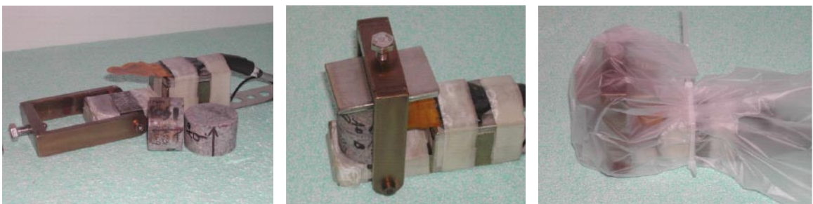
Figure 3-2. Specimens prior to mounting (left), mounted in stainless sample holder (middle), and sample holder with mounted specimens wrapped in plastic (right).
