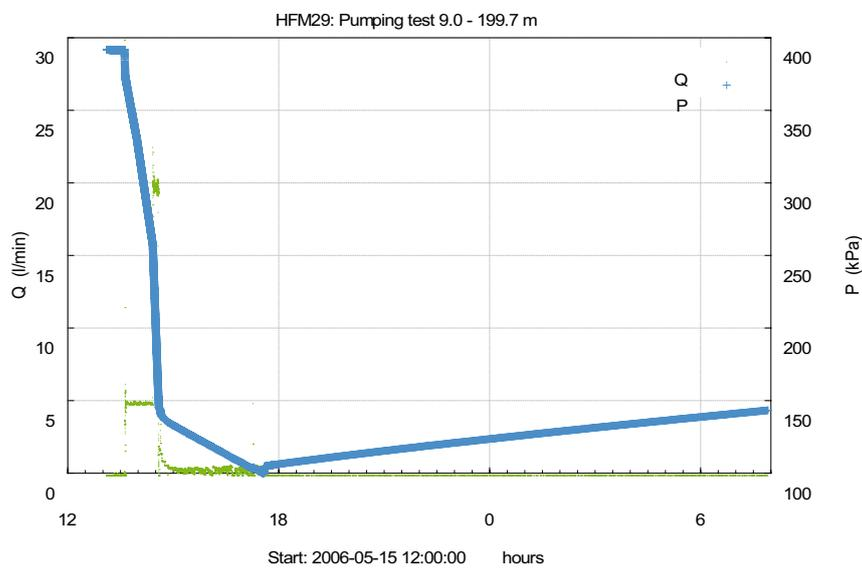
**Figure A2-1.** Linear plot of flow rate ( $Q$ ) and pressure ( $P$ ) versus time during the open-hole pumping test in HFM29.
