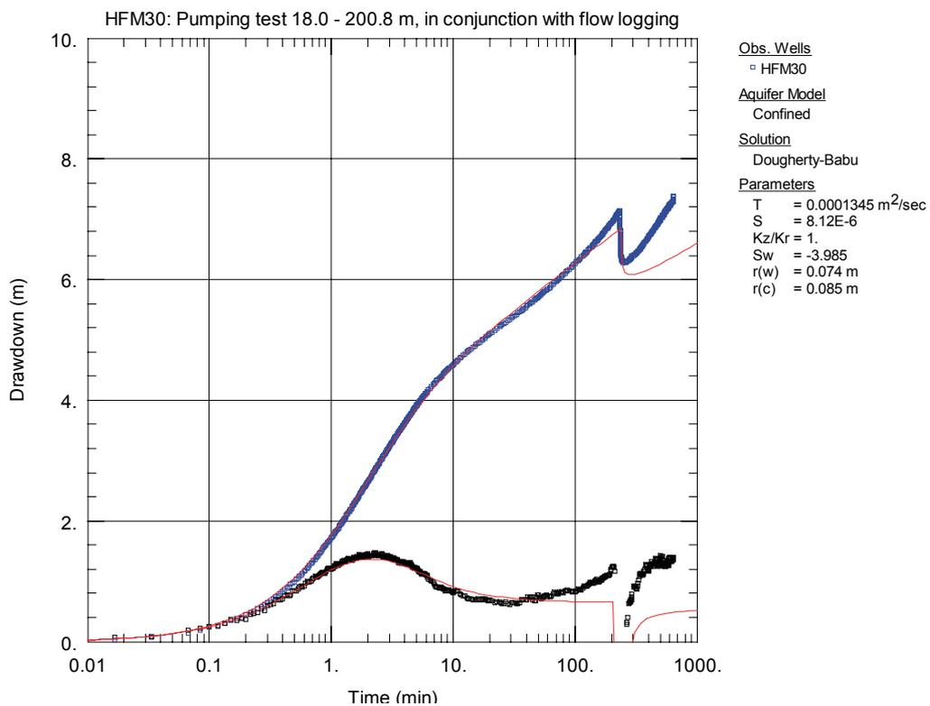
**Figure A2-7.** Lin-log plot of drawdown (blue □) and drawdown derivative (black +) versus time during the open-hole pumping test in HFM30.
