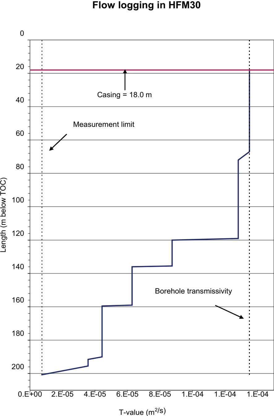
**Figure 6-4.** Calculated, cumulative transmissivity along the flow logged interval of borehole HFM30. The total borehole transmissivity was calculated from the pumping test during flow logging.
