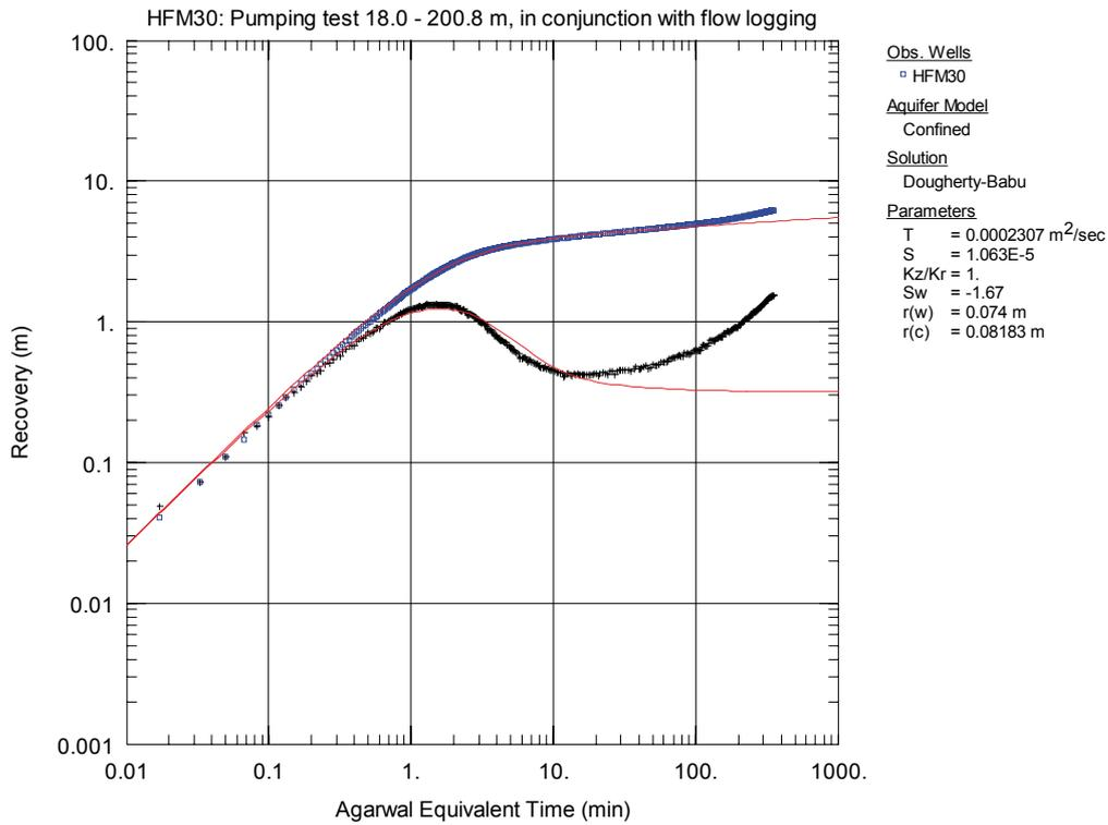
**Figure A2-8.** Log-log plot of pressure recovery (blue □) and -derivative (black +)  $dsp/d(\ln dte)$  versus equivalent time ( $dte$ ) from the open-hole pumping test in HFM30.
