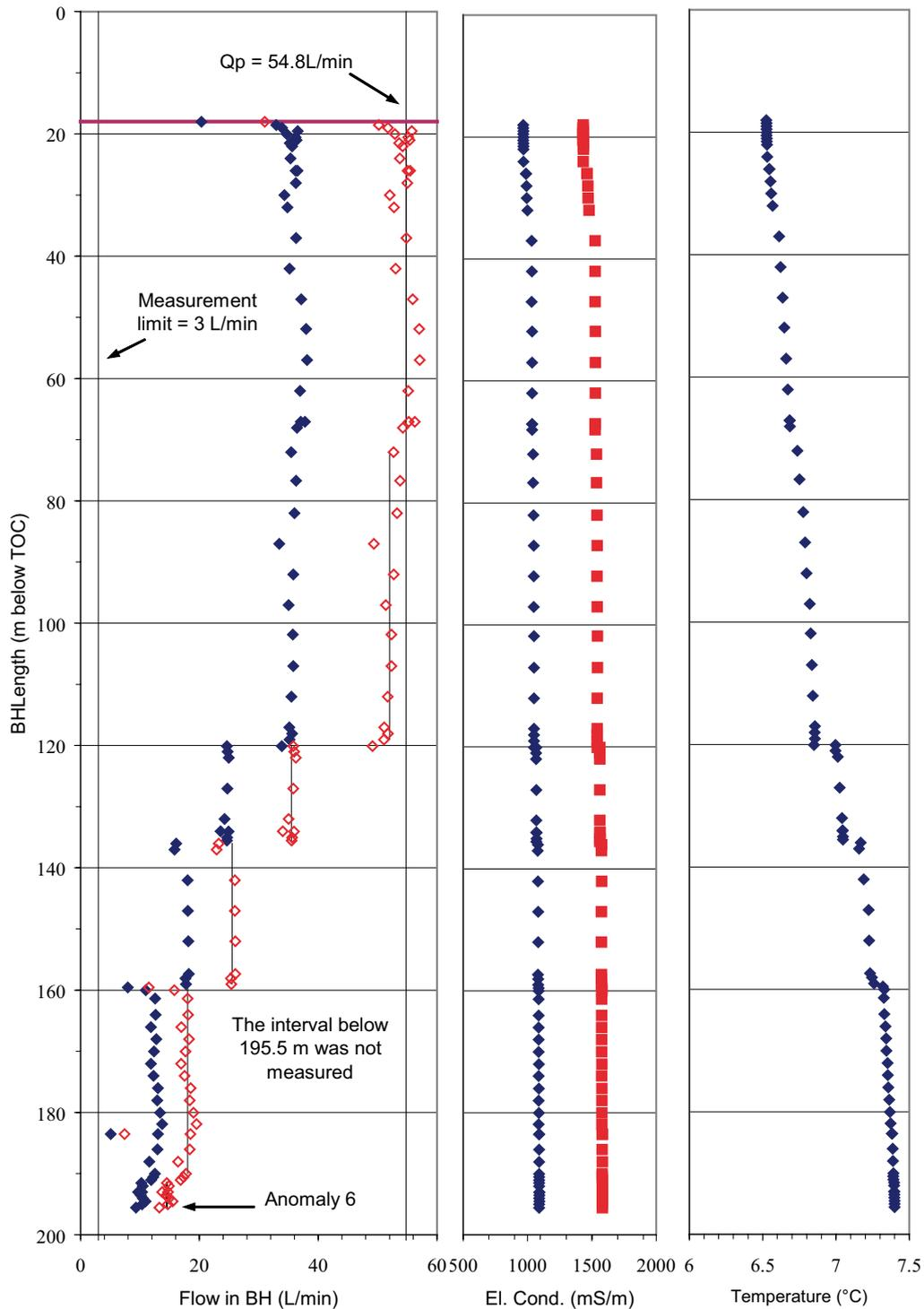
**Figure 6-3.** Measured (blue) and corrected (red) inflow distribution together with measured (blue) and temperature compensated (red) electrical conductivity and temperature of the borehole fluid along borehole HMF30 during flow logging. (Total logged interval.)
