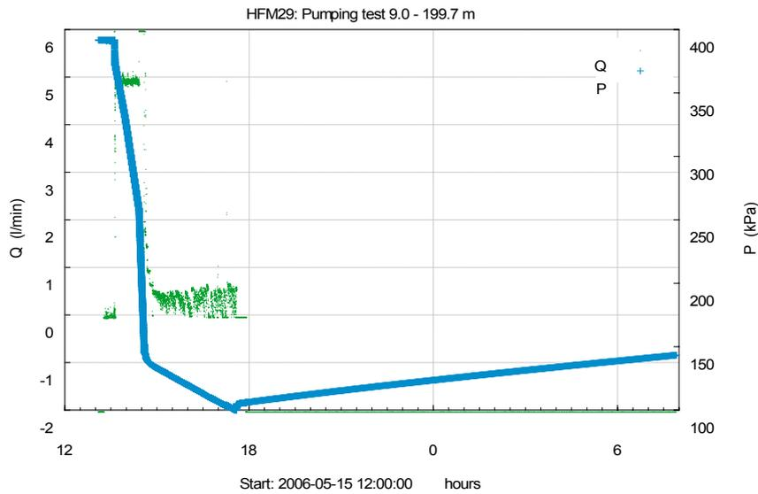
**Figure A2-2.** Linear plot of flow rate ( $Q$ ) and pressure ( $P$ ) versus time, with a more detailed scale for the flow rate ( $Q$ ), during the open-hole pumping test in HFM29.
