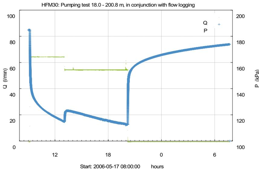
**Figure A2-5.** Linear plot of flow rate ( $Q$ ) and pressure ( $P$ ) versus time during the open-hole pumping test in HFM30 in conjunction with flow logging.
