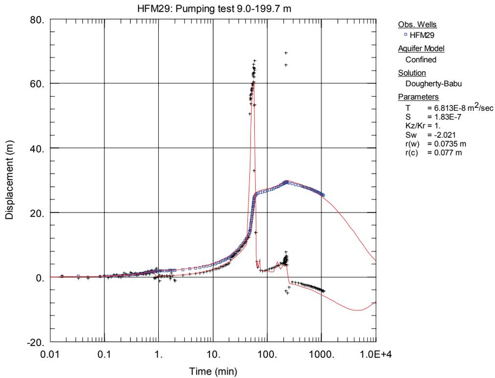
**Figure A2-4.** Lin-log plot of drawdown and recovery (blue □) and drawdown and recovery derivative (black +) versus time during the open-hole pumping test in HFM29.
