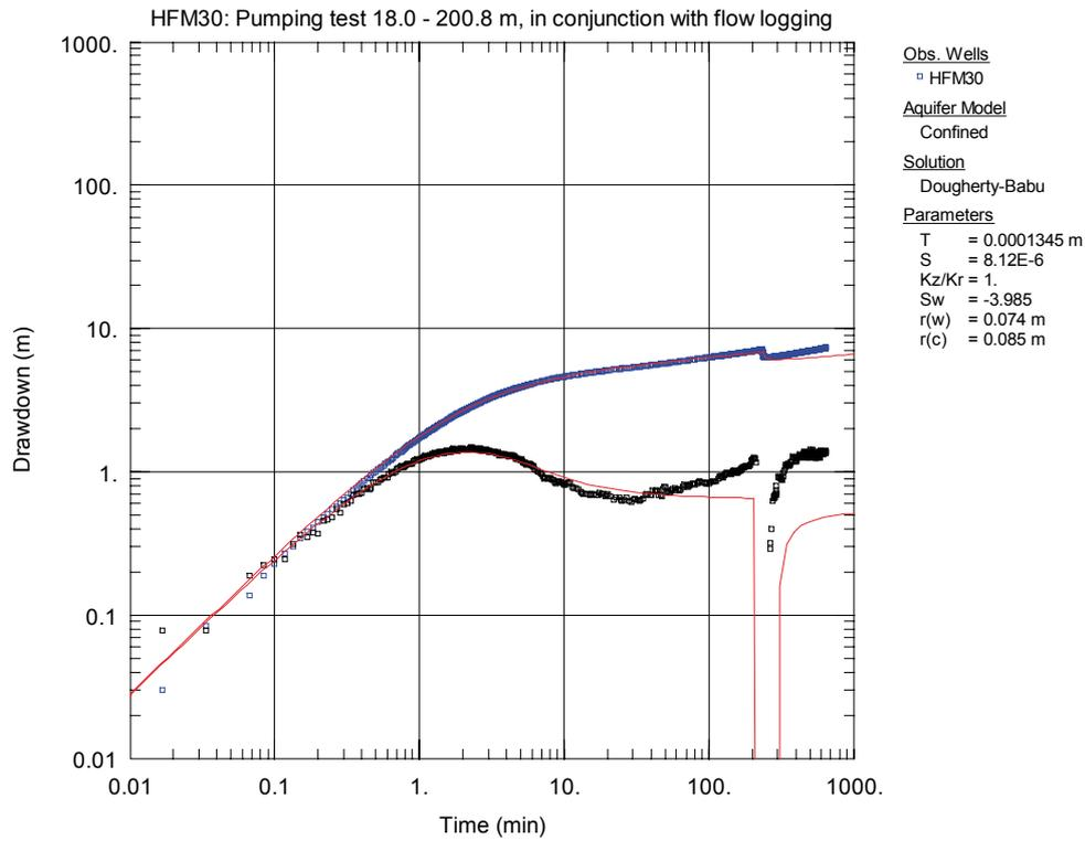
**Figure A2-6.** Log-log plot of drawdown (blue □) and drawdown derivative (black +) versus time during the open-hole pumping test in HFM30.
