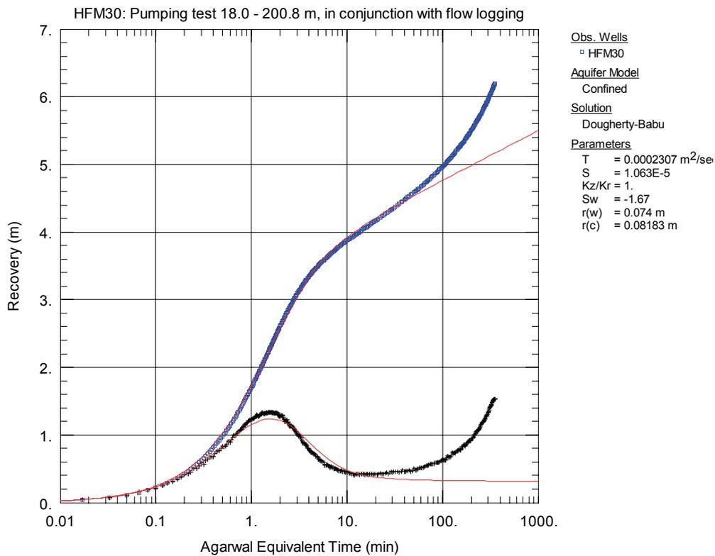
**Figure A2-9.** Lin-log plot of pressure recovery (blue □) and -derivative (black +)  $dsp/d(\ln dte)$  versus equivalent time ( $dte$ ) from the open-hole pumping test in HFM30.
