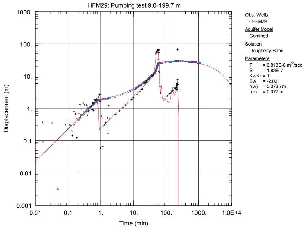
**Figure A2-3.** Log-log plot of drawdown and recovery (blue  $\square$ ) and drawdown and recovery derivative (black  $+$ ) versus time during the open-hole pumping test in HFM29.
