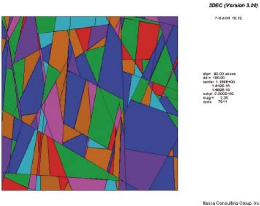
Figure 3-3. Contact points along fractures in the 3DEC model.
