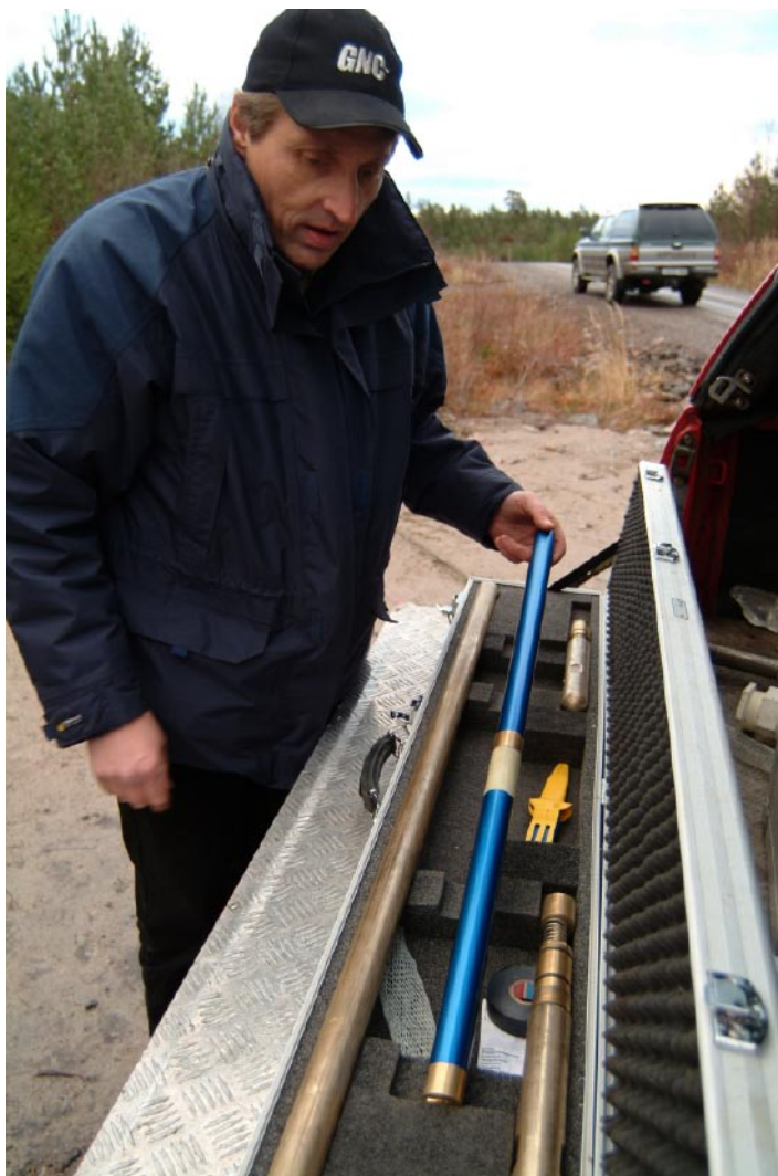
Figure 3-4. Deviation measurements in HFM26 were performed with a Flexit Multi-shot (magnetic) equipment.
