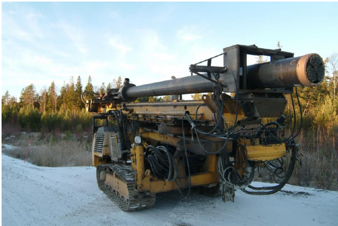
Figure 3-1. The Nemek 710 percussion drilling machine employed for drilling the percussion boreholes HFM25, HFM26, HFM27 and HFM29.
