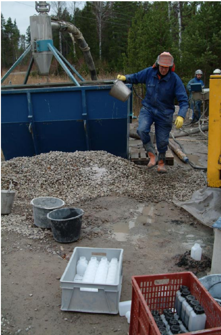
Figure 4-2. Sampling of drill cuttings from the penetrated bedrock in HFM27.
