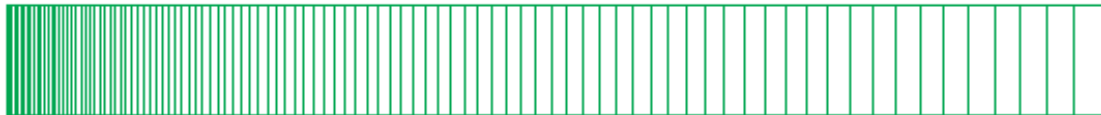
Figure 5-1. 10 m element mesh with 100 elements for the modelling of long small pipes in bentonite. Axial symmetry around a vertical axis 1 cm left of the mesh.
