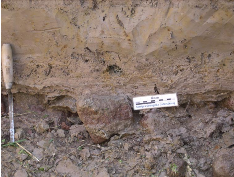
Figure 5-5. In most of the trenches the sandy-silty glaciofluvial deposits searched for were missing. In this section, at Mölstad close to Mönsterås (E4 in Figure 1-1), fairly thin varved glacial clay rests directly on top of coarse glaciofluvial gravel.
