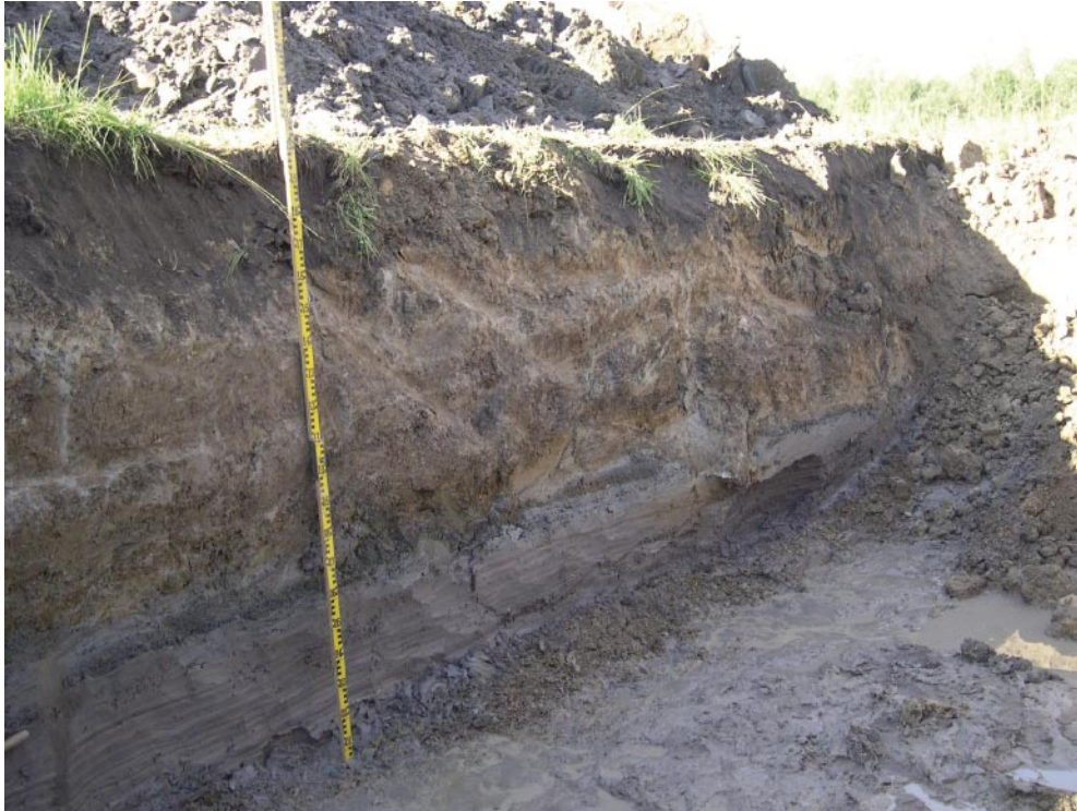
Figure 5-7. Similar to Högalid (Figure 5-6) the diamict deposits at Dockrössle (E11 in Figure 1-1) is divided by a thin sand layer but here the two beds have a similar, mainly silty-clayey composition. Coarser clasts and sheared lenses of sand, gravel and laminated clay-silt float in a silty-clayey matrix. The contact with underlying laminated silt and clay is gradual and the bottommost parts of diamicton have an increased content of silt and clay.
