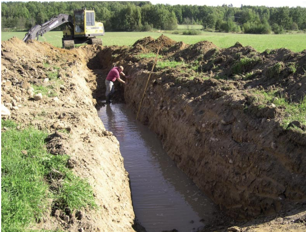
Figure 5-14. Trench dug at Träda (E10 in Figure 1-1) along the Påskallavik esker some 30 km west of Simpevarp. Although raised above the sea before 12,000 years BP and, thus, entirely water-logged during only some 1,500 years, the silty deposits at depth have to some degree, due to a fairly high groundwater table, remained susceptible to seismically induced deformation.
