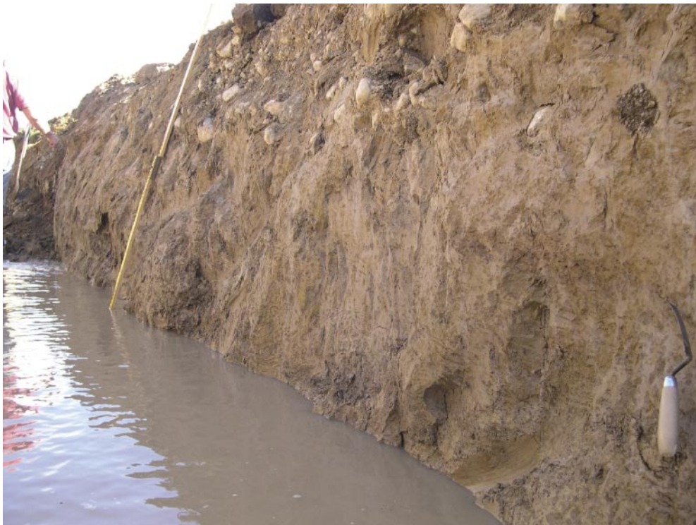
Figure 5-8. At Träda (E10 in Figure 1-1) along the Påskallavik esker a stony diamicton with silty matrix covers structureless silt, downwards gradually merging into folded and, finally, undisturbed thin-bedded silt.
