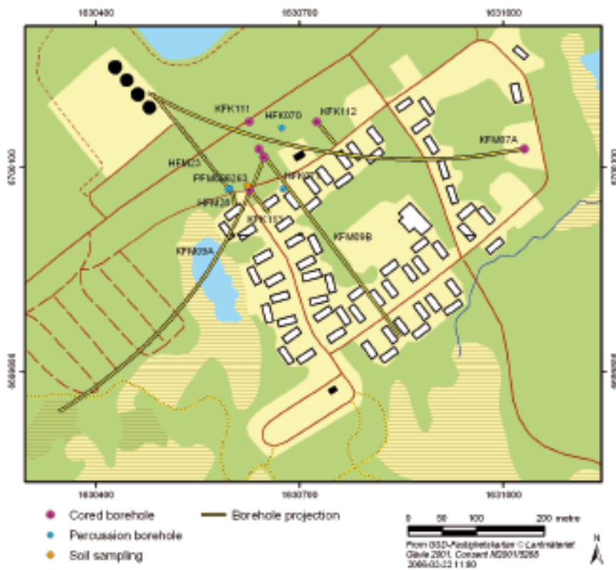
Figure 1-2. Location and projection on the horizontal plane of the cored borehole KFM09B and the surrounding boreholes at drill sites DS9 and DS7.
