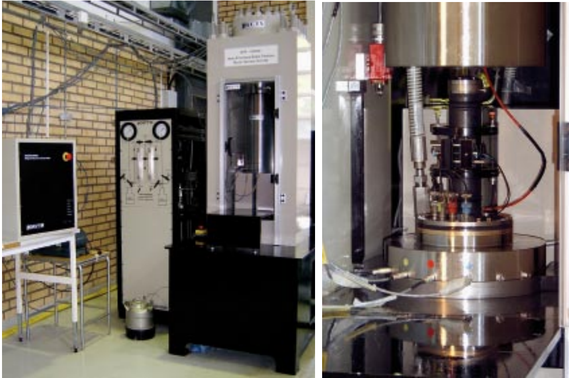
Figure 3-1. Left: Digital controller unit, pressure cabinet with cell pressure intensifier and oil reservoir inside, and the load frame with closed cell (pressure vessel). Right: Bottom of the cell is lowered. The specimen is instrumented and ready for inserting in the cell.
