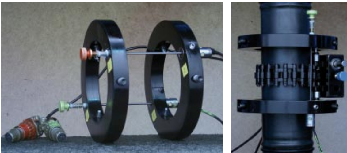
Figure 3-2. Left: Rings and LVDTs for axial deformation measurement. Right: Specimen and loading platens sealed with a rubber membrane. Devices for axial and circumferential deformation measurements are attached.
