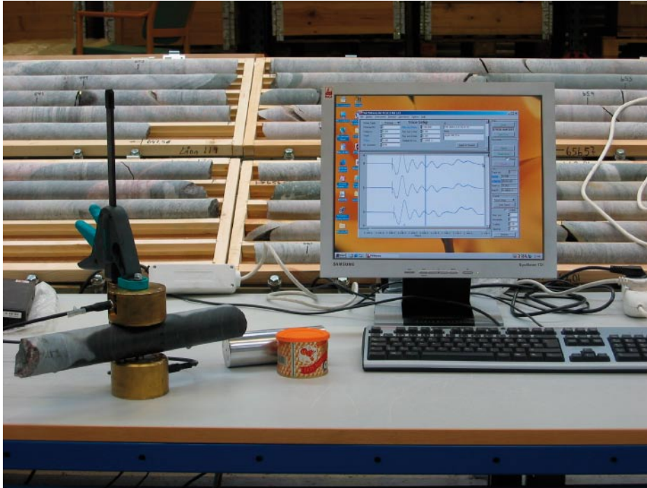
Figure 3-2. NGI's equipment set-up for measuring acoustic P-wave travel time transverse a drill core.
