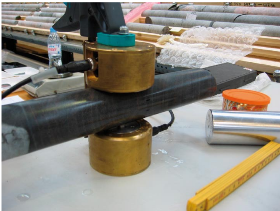
Figure 3-1. Detail of NGI's apparatus for measuring acoustic P-wave travel time transverse a foliated drill core. The aluminium cylinder for calibration of the device is on the right.
