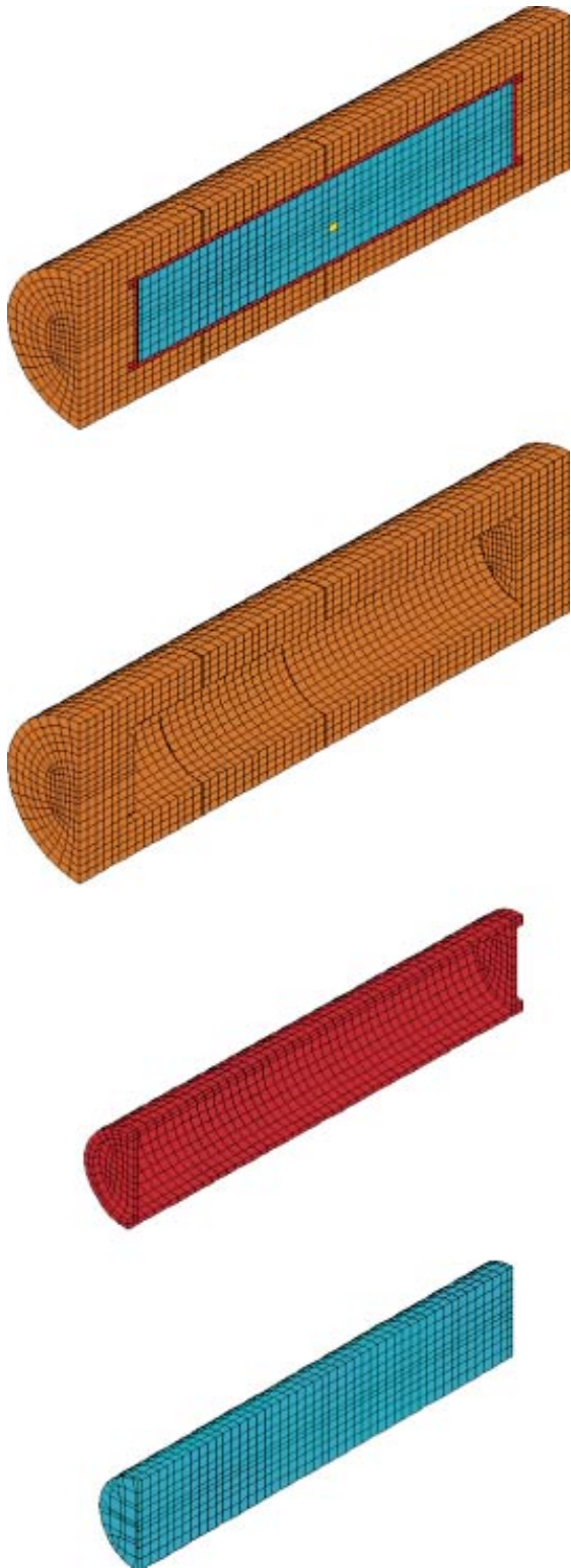
Figure 4-1. Element mesh (from top to bottom) of the entire model, the bentonite buffer, the copper canister and the cast iron insert. The location of the shear planes are marked in the bentonite.
