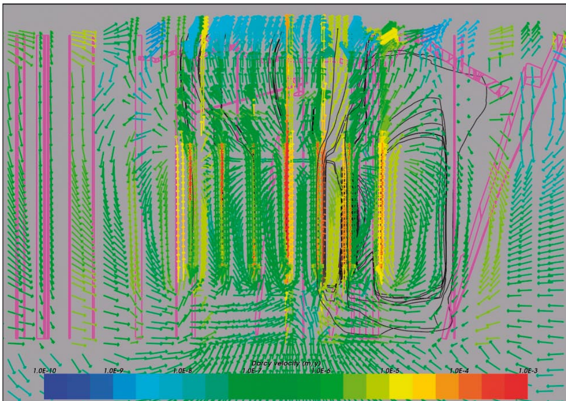
Figure 3-25. Case 9. Close-up view of a vertical section showing Darcy velocity vectors. Flow paths are superimposed for illustration. Time = 100 years.
