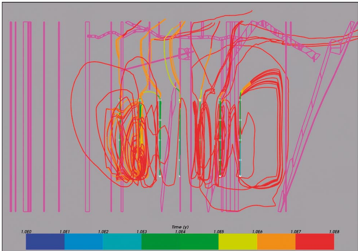
Figure 3-26. Case 9. Vertical section showing flow paths coloured by travel time along the paths. Particle release time = 10 years.
