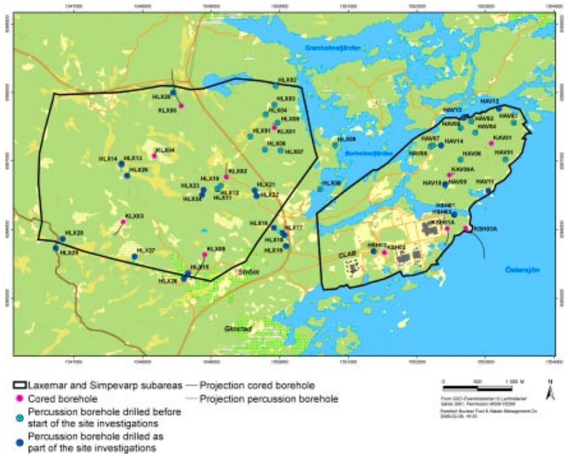
Figure 1-3. Overview map of core-drilled and percussion-drilled boreholes in the Laxemar and Simpevarp subareas at stage model version Laxemar 1.2. Location of the core-drilled boreholes with new site investigation data available for model version Laxemar 1.2: KSH01A, KSH02, KSH03A, KAV01, KLX02, KLX03, KLX04 and KAV04A,B.
