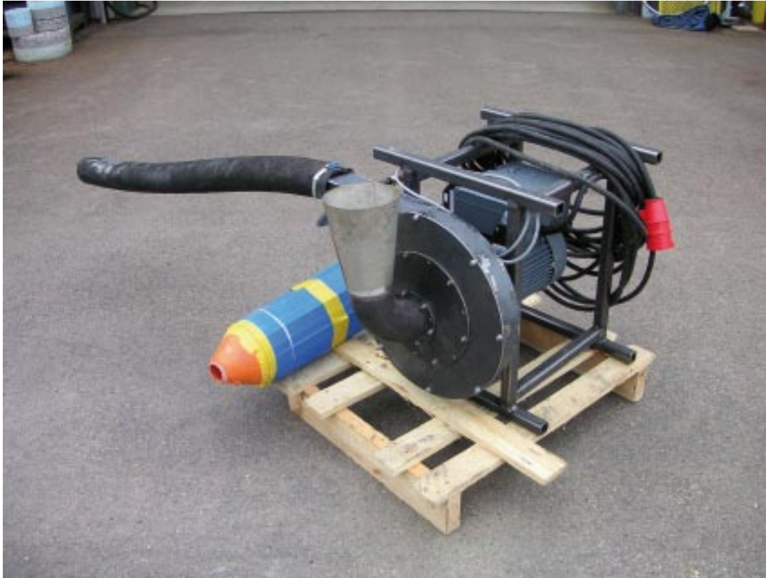
Figure 5-8. Test equipment for placing pellets “pellet thrower”.
