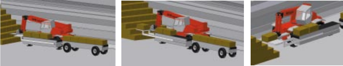
Figure 5-5. Loading of blocks to the placement tool.
