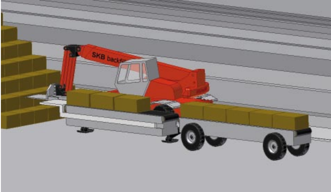
Figure 5-4. Block placement equipment (left) and transport unit (right) at the backfilling front.
