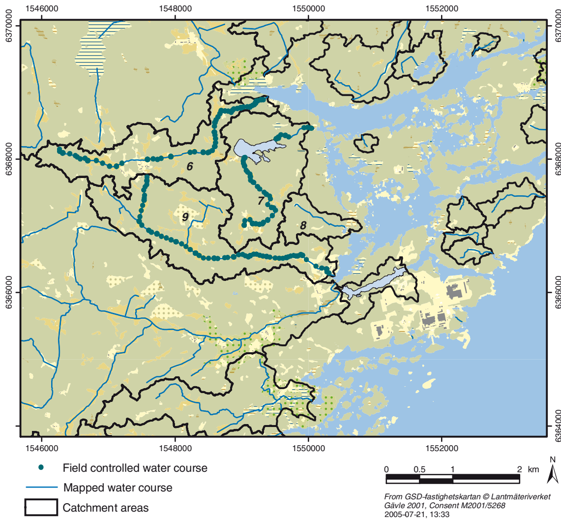
Figure 4-8. Map showing the surveyed main watercourses in catchment areas 6 (Mederhultsån), 7 (Kåreviksån) and 9 (Ekerumsån). The surveying also included a tributary to Ekerumsån /Strömgren 2006/. Pistlanbäcken in catchment area 8 has not been surveyed.
