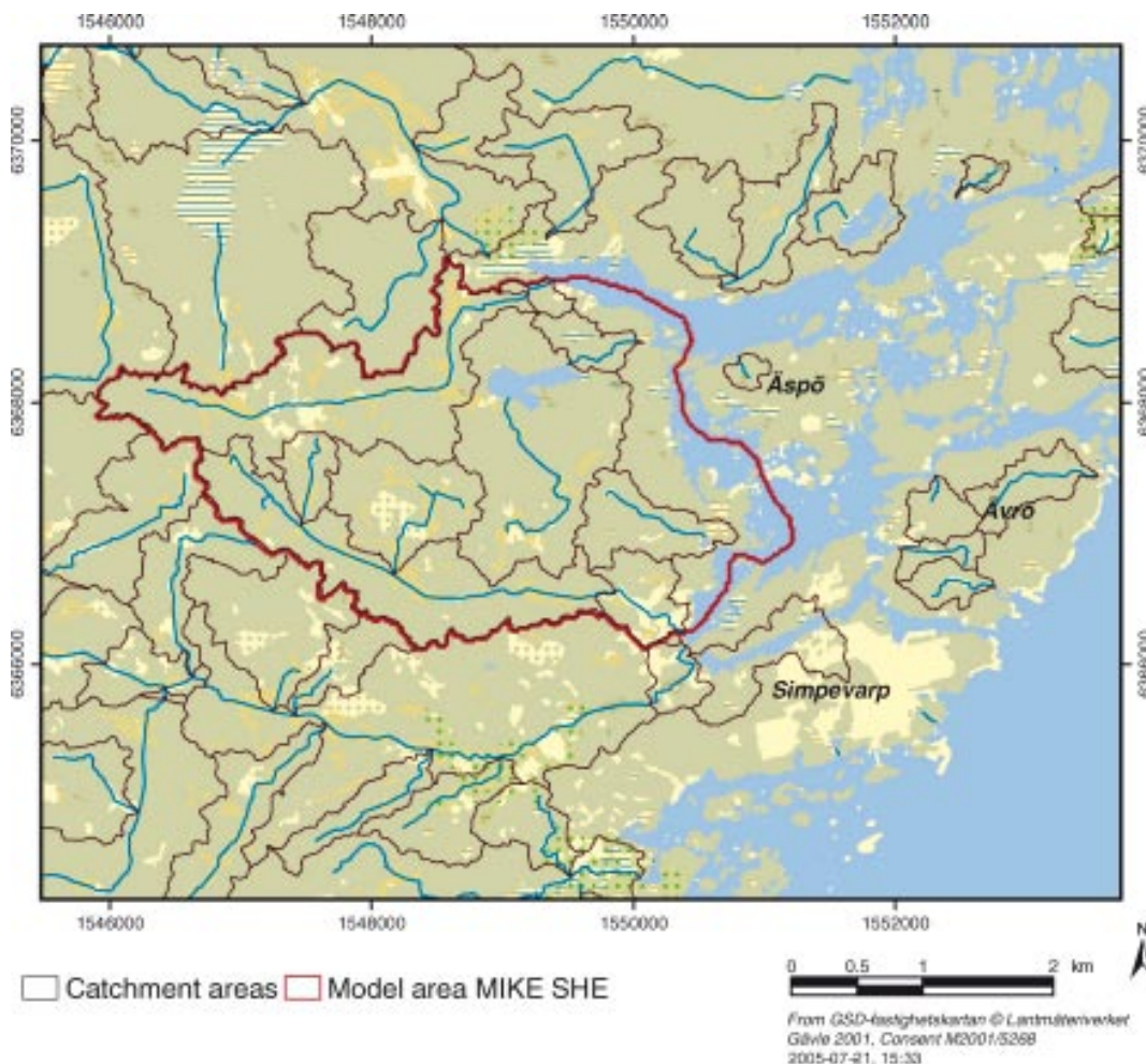
Figure 4-5. Catchment area boundaries (black lines) /Brunberg et al. 2004/ and the boundary of the MIKE SHE-MIKE 11 model area (red line). Note that the model area also includes the areas along the coastline, outside (downstream) of catchment areas 6-9.
