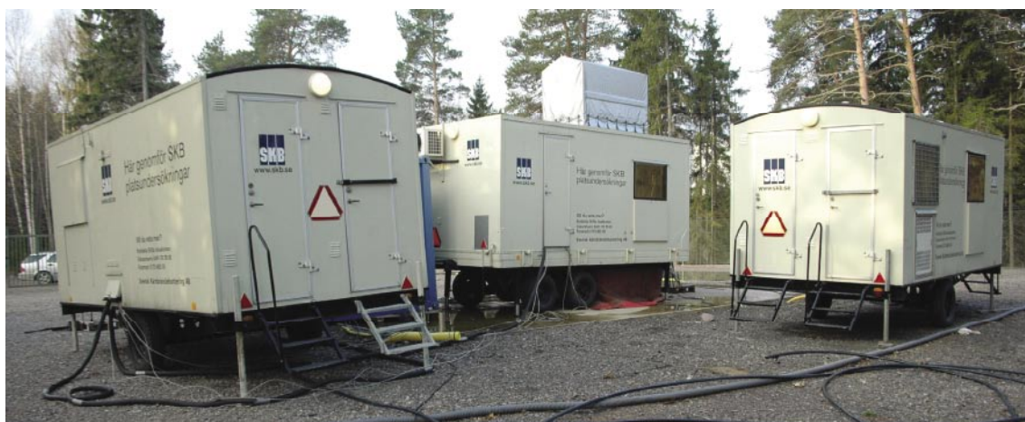
Figure 4-1. The mobile field laboratory units at KFM08A; from the left a computer unit (MYC 2), container for collecting the water from the borehole, hose unit with downhole equipment (S2) and a spare unit for computer work (MYC3), November 2005.
