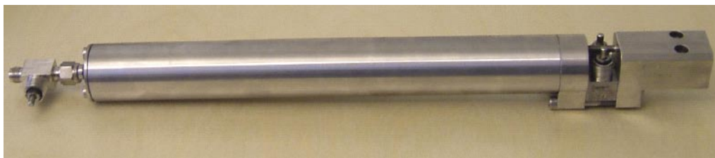
Figure A7-3. SKB stainless steel sampling cylinder (left: piston side, right: mounting adapter side).
