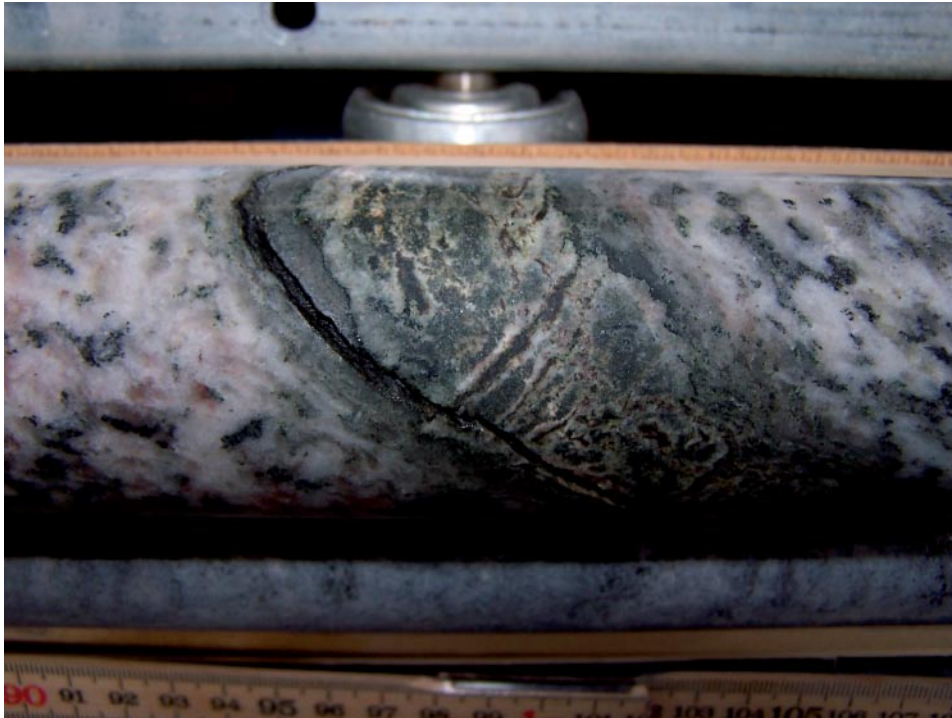
Figure 5-4. Reactivated skarn alteration in KFM01C, 113.98–114.02 m.
