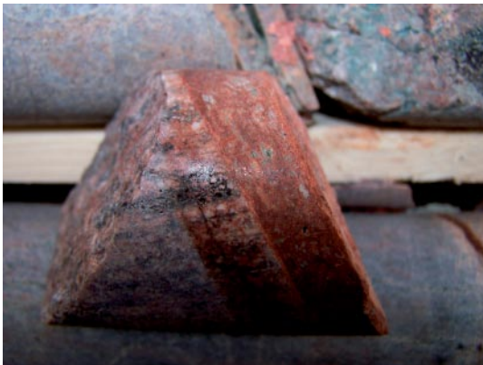
Figure 5-2. Laumontite-sealed breccia, KFM01C, probably the one at 33.60 m borehole length.
