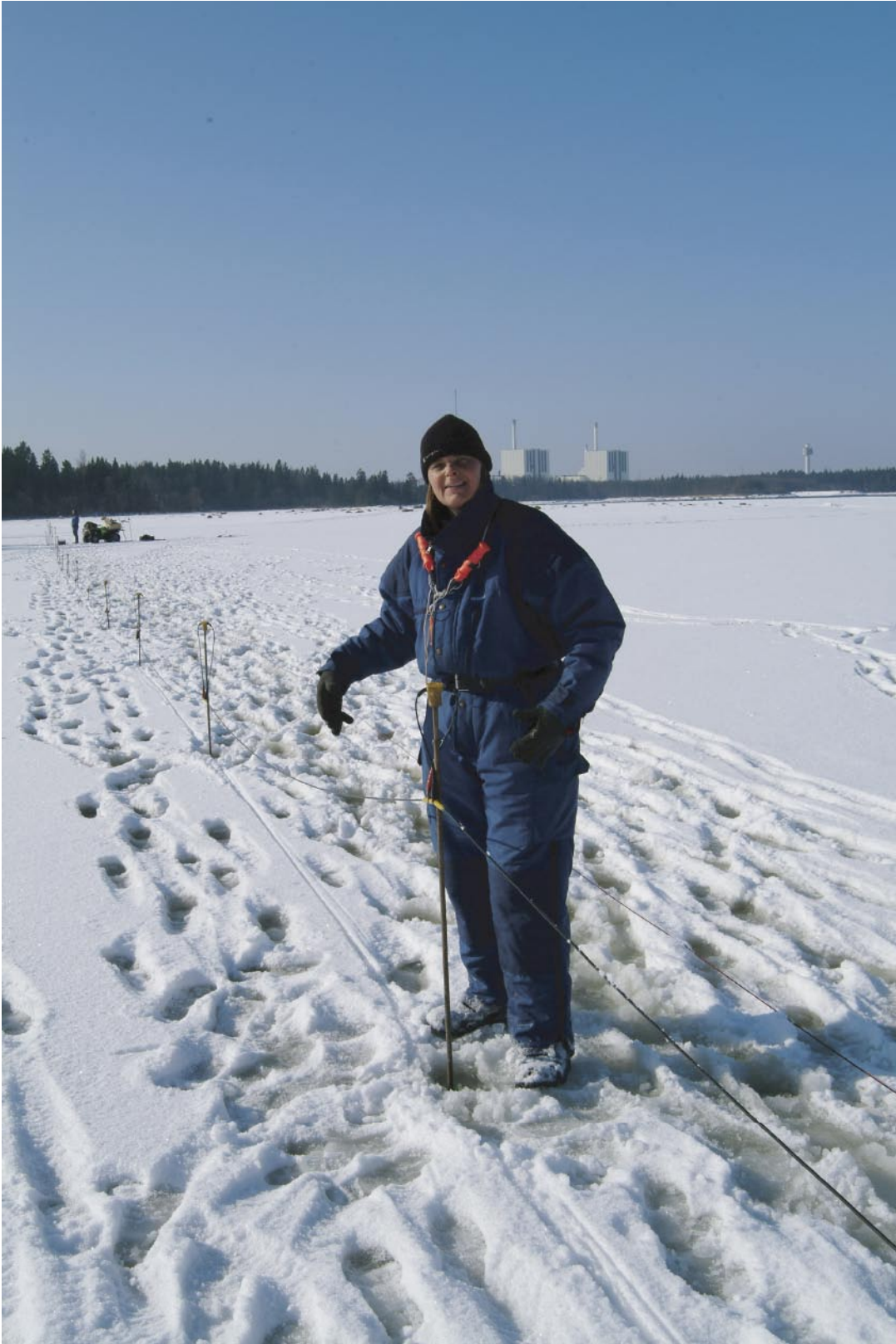
Figure 3-1. Some of the profiles were measured during the winter on the lakes. The geophones were placed on top of long steel-stakes, pressed into the lake sediments.
