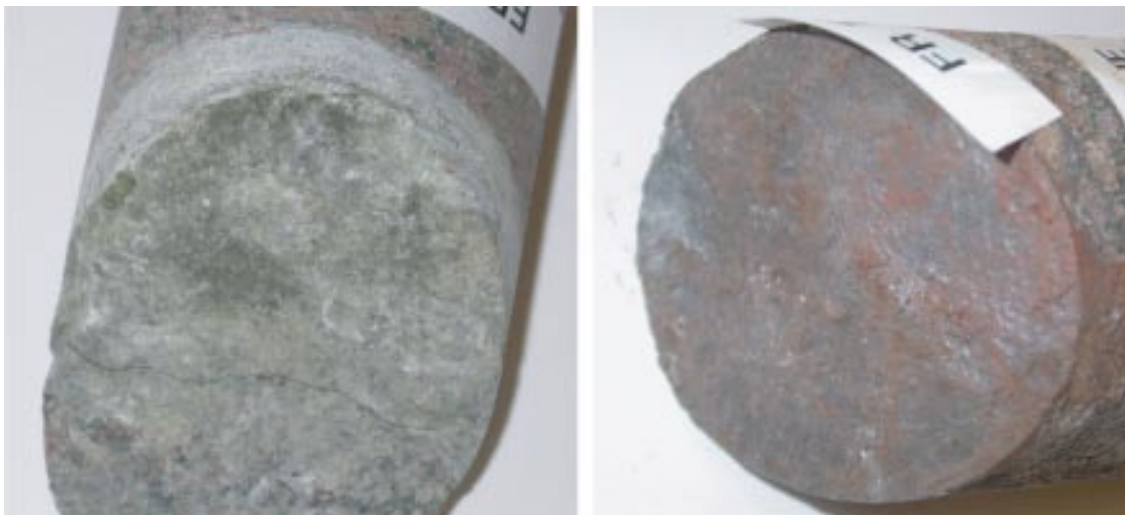
Figure 2-3. Fracture planes with chlorite + calcite and prehnite (left), and chlorite + calcite and hematite (right).
