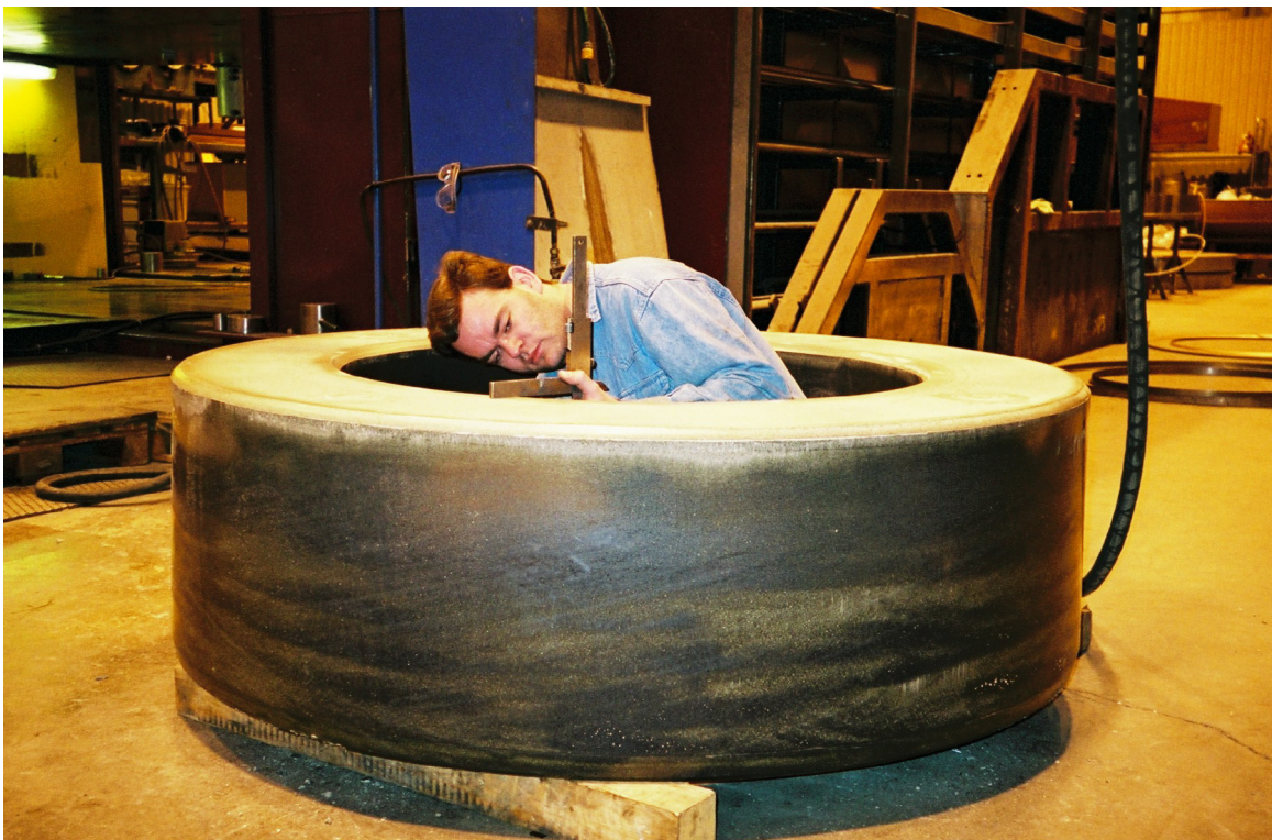
Figure 2-7. A bentonite ring after completed compaction and dismounting.
