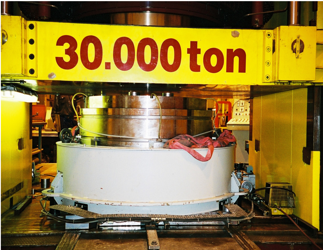
Figure 2-6. Compaction of a bentonite block at Hydroweld in Ystad.
