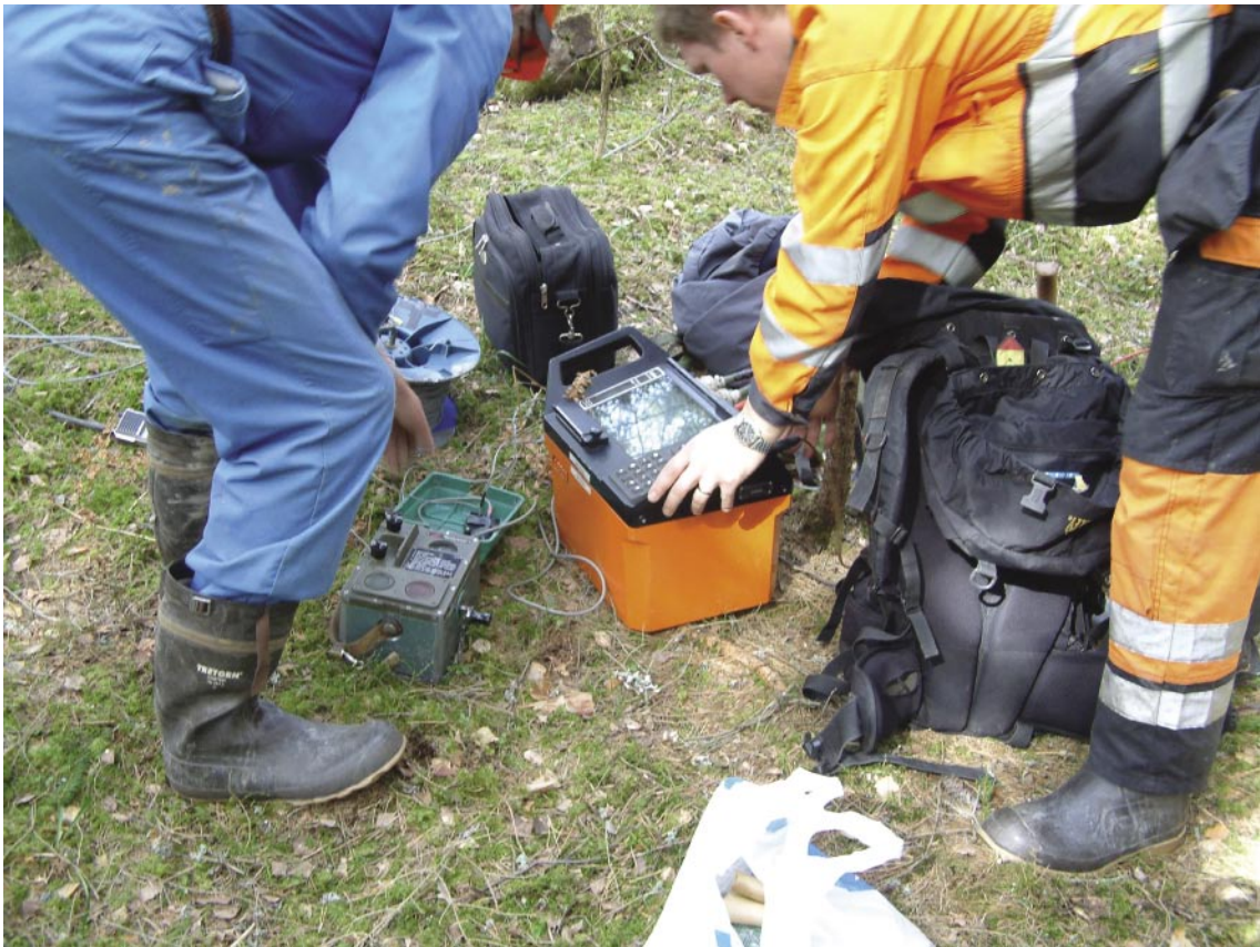
Figure 3-1. The recording instrument, ABEM Terraloc MK6.
