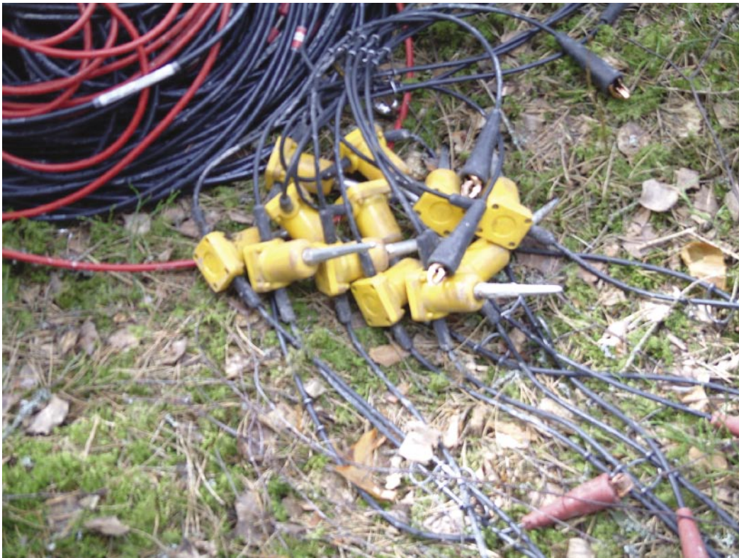
Figur 4-1. Geophones used during the survey.
