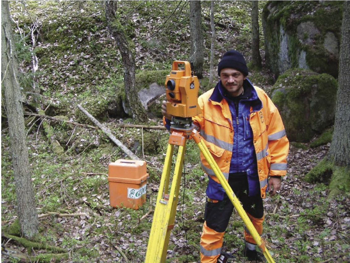
Figure 4-2. Line survey with Total station.
