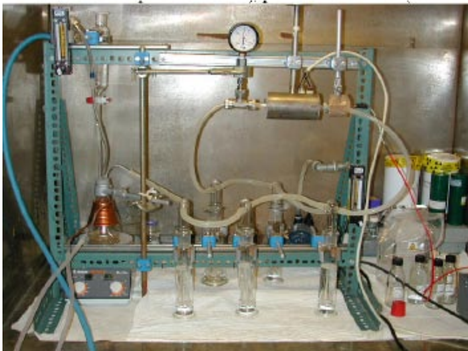
Figure 3-2. System setup for processing samples of spent ion exchange resins. Three-way valves, disconnecting the two bottles used for absorbing inorganic species after completed acid stripping, are missing in the photo.
