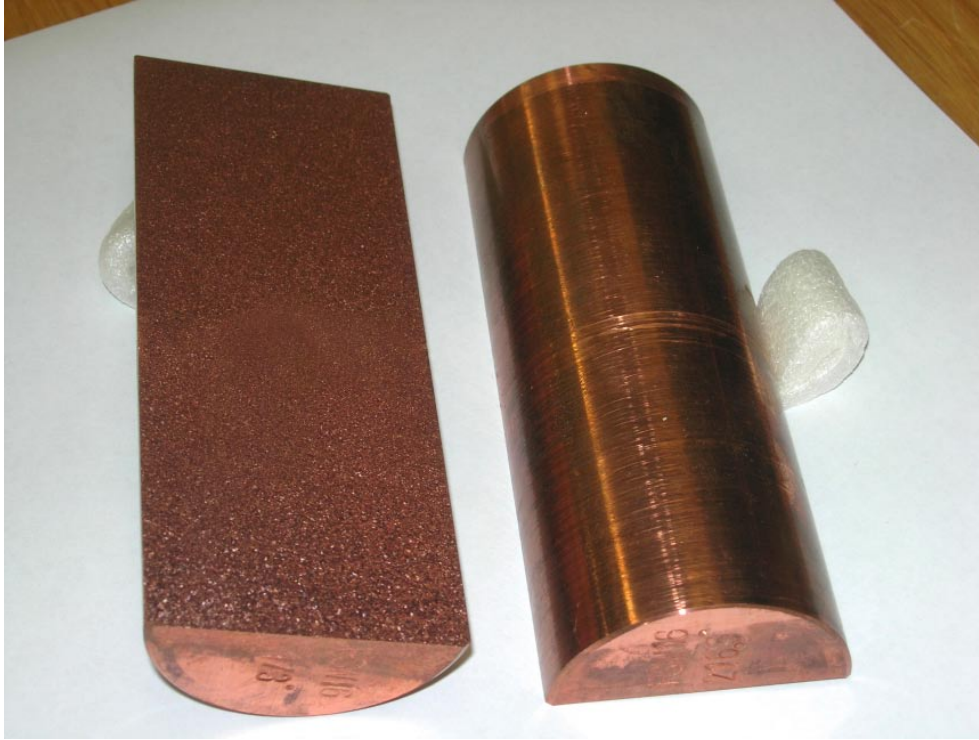
Figure A5-1. Core for destructive evaluation of joint line hooking.
