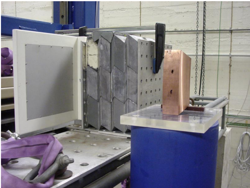
Figure A5-6. Display detail of flat panel detector and Cu sample on the scanner table. The electronic part of the detector was shielded against X-ray radiation with 20 cm of lead.
