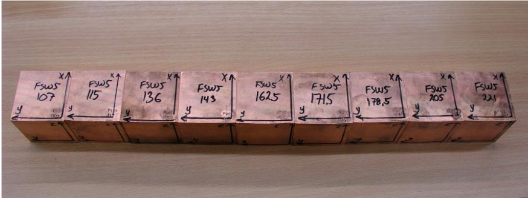
Figure A5-3. Copper cubes for destructive evaluation of wormholes.
