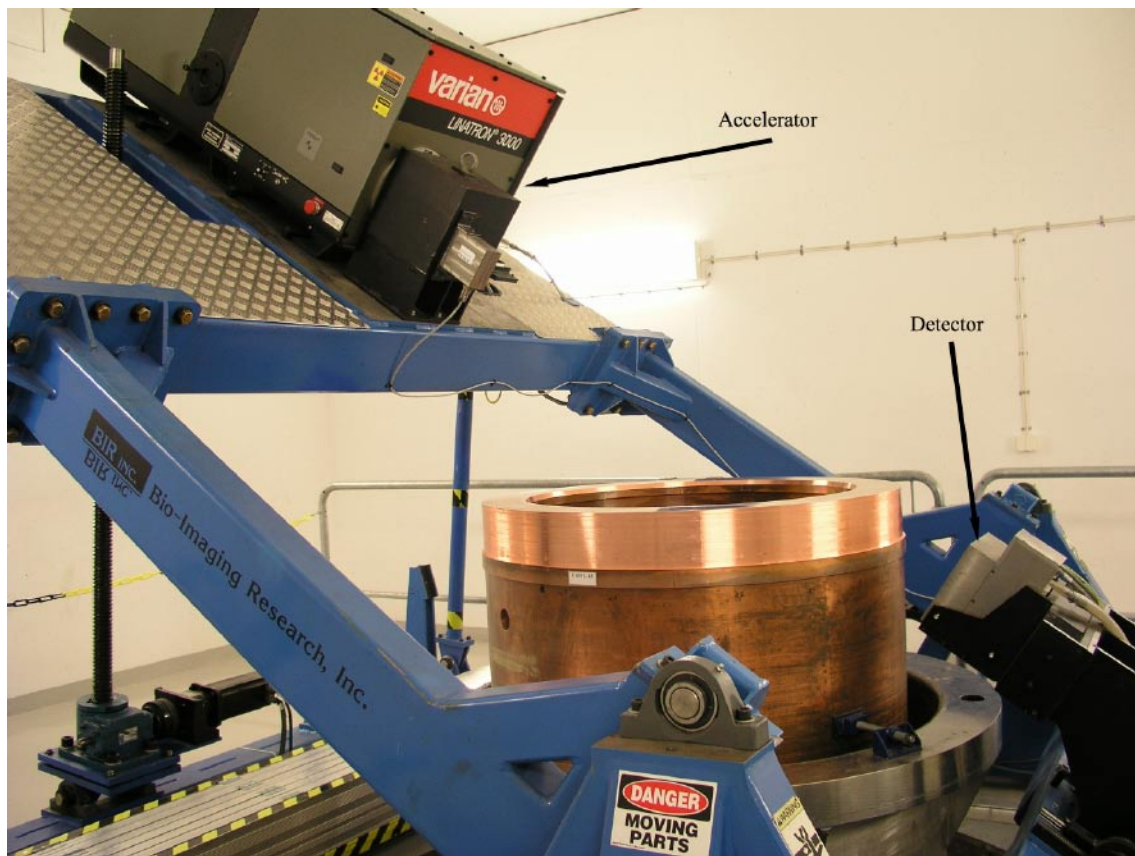
Figure 5-1. X-ray machine for testing of the copper canister's sealing weld.
