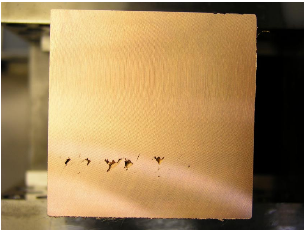
Figure A5-4. Photograph at 6.2 mm depth of wormholes in weld FSW5.
