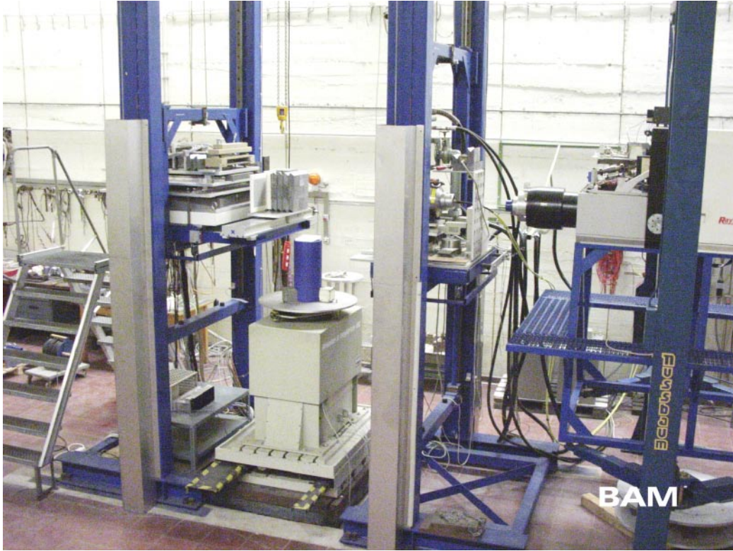
Figure A5-5. Multi-purpose-Tomograph of BAM with the LINAC X-ray source at right and the flat panel detector at left.
