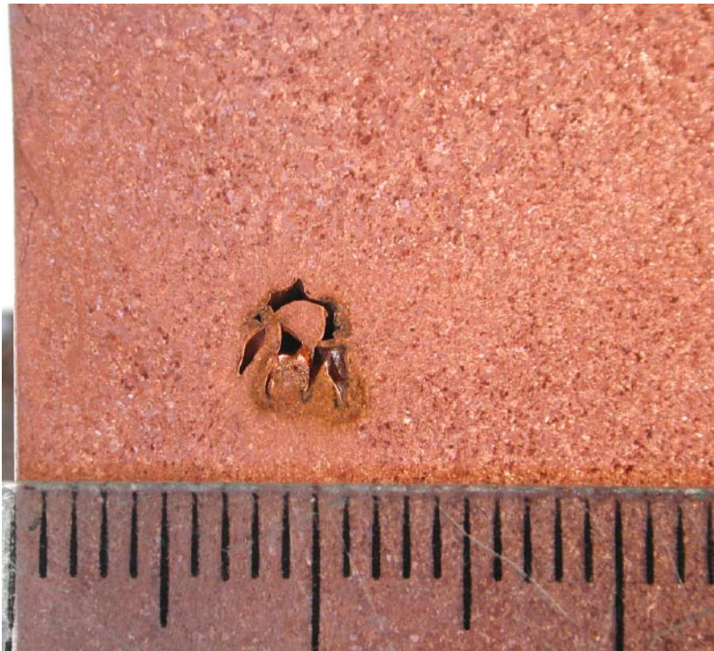
Figure 6-4. Macrospecimen of volumetric wormhole.
