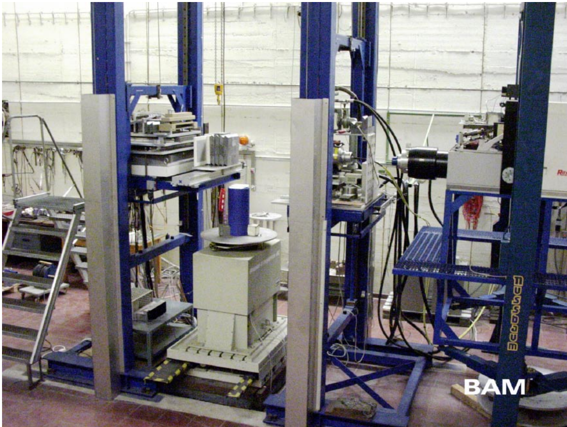
Figure 5-5. Multi-purpose-Tomograph of BAM with the LINAC X-ray source at right and the flat panel detector at left.
