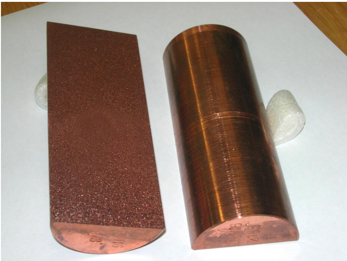
Figure 5-1. Core for destructive evaluation of joint line hooking.
