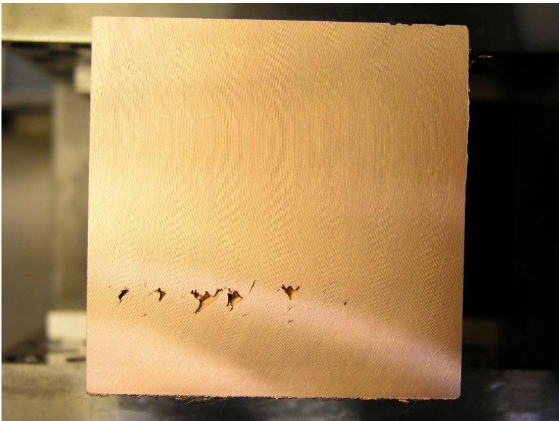
Figure 5-4. Photograph at 6.2 mm depth of wormholes in weld FSW5.
