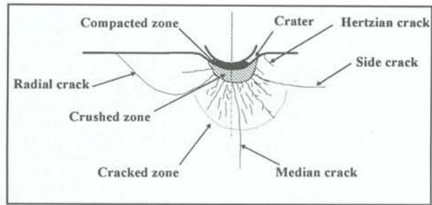
Figure 13-8. Conceptual view of cracks in rock caused by mechanical excavation.
