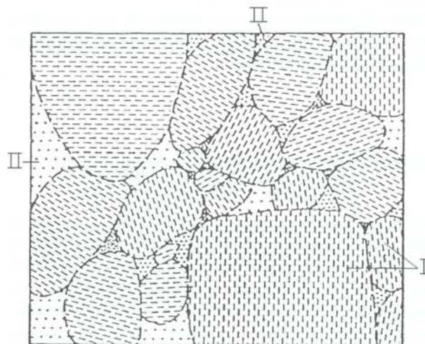
Figure 15.2-1. Basic pattern of granules in highly compacted bentonite clay:
