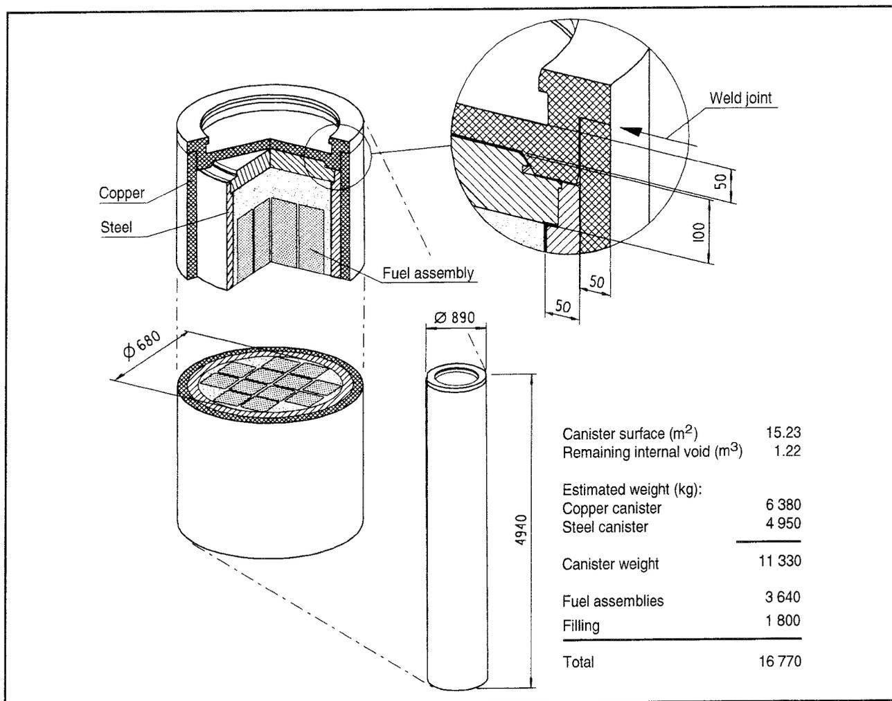
Figure 14-4. Copper/steel canister with BWR assemblies.
