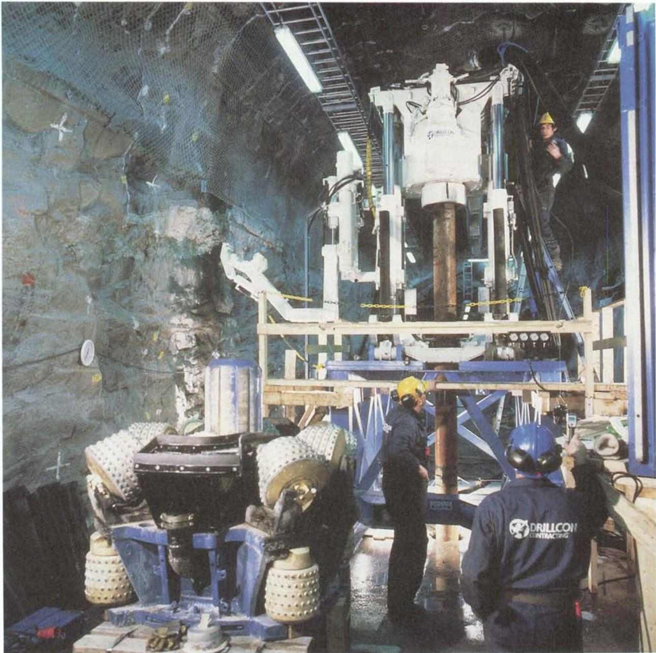
*Figure 13-5. Test of boring full-scale vertical deposition holes. The boring machine was placed on a frame in order to provide space for mounting the cutterhead.*
