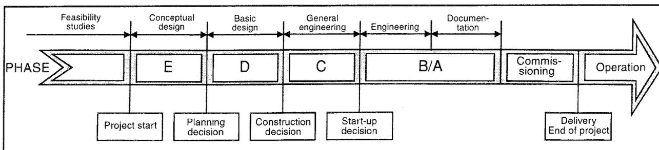
Figure 13-3. Schematic illustration of the repository design process.
