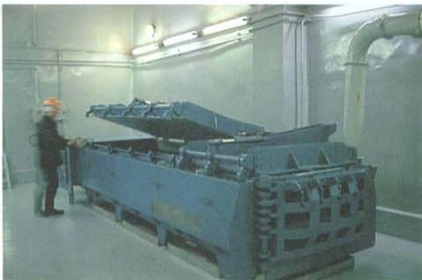
*Figure 10-2. Compactor for low level waste, delivered to Ignalina NPP.*
