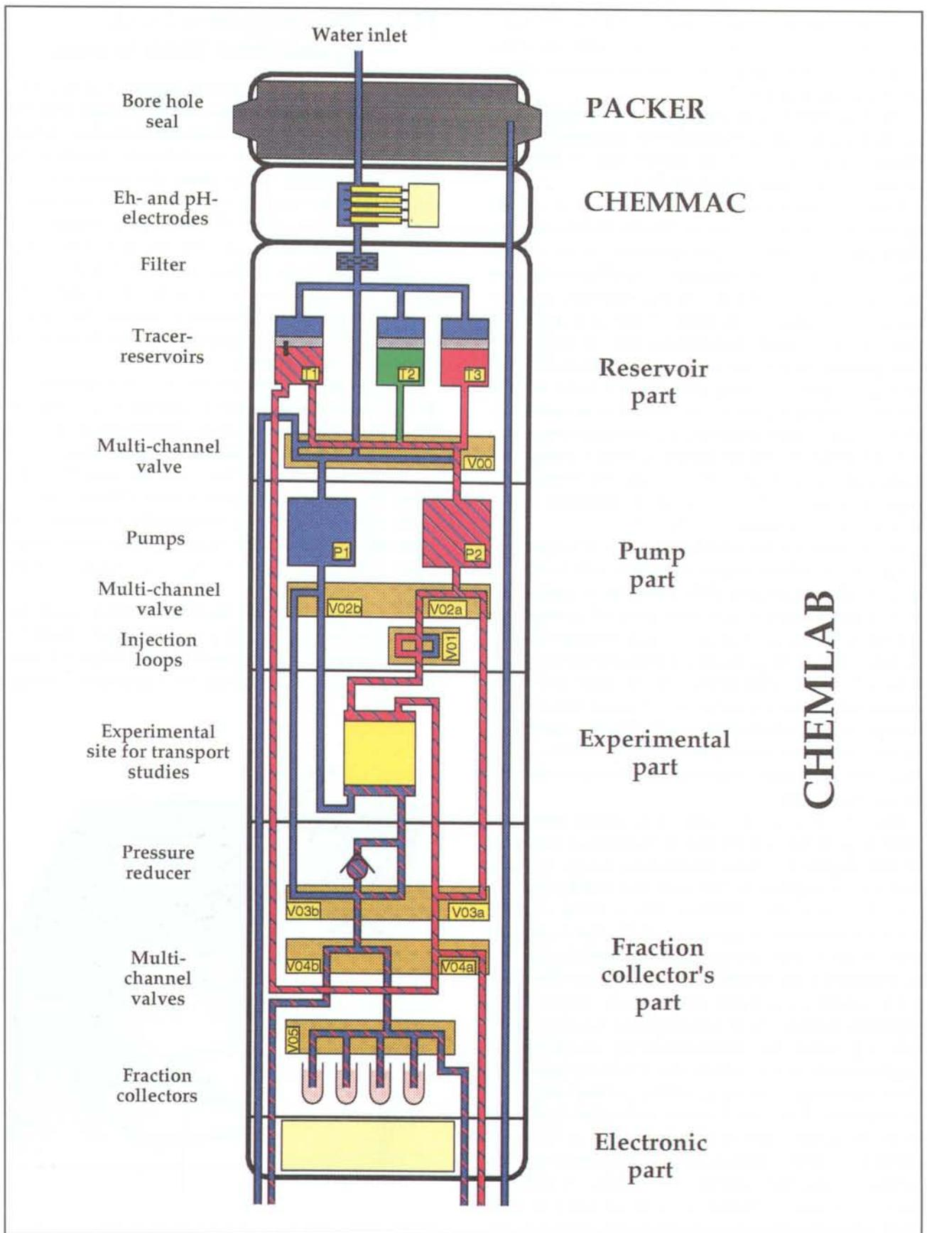
Figure 17-4. Schematic illustration of the CHEMLAB probe.
