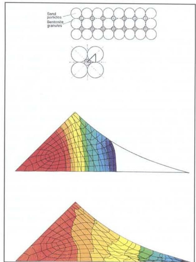
Figure 15.2-2. Preliminary material calculation of the maturation rate of bentonite granule assemblage in bentonite/ballast mixture. Upper: Schematic microstructure. Centre: Early stage with a large part of voids still unfilled. Lower: Late stage with a small part of voids unfilled. Red is high density, yellow intermediate density and blue very low density.
