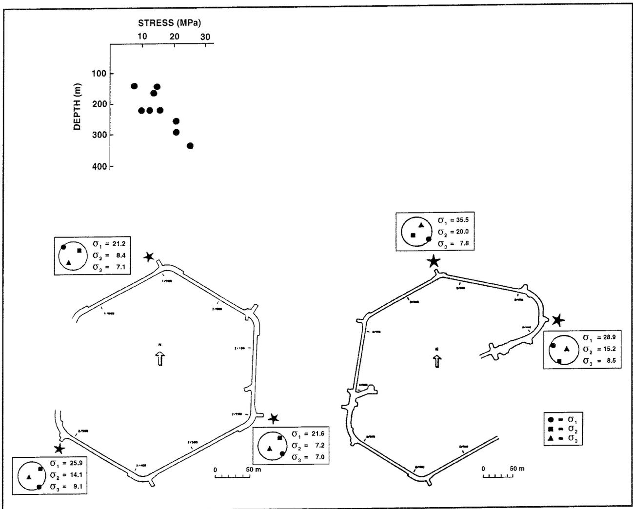
**Figure 17-2.** Compilation of stress measurement results. Overall trend with depth for maximum principal stress (upper) and data from recently completed tests (lower).
