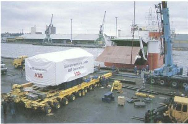
*Figure 3-2. Loading of a 400 tonnes generator stator on board M/S Sigyn.*
