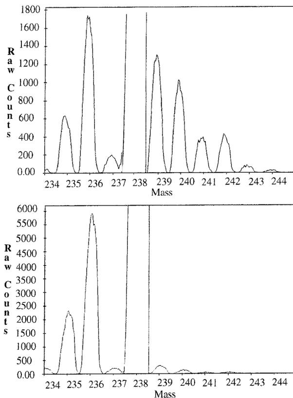
**Figure 15.1-1.** Actinide spectra from specimens from the high burnup end of the stringer fuel rod.
