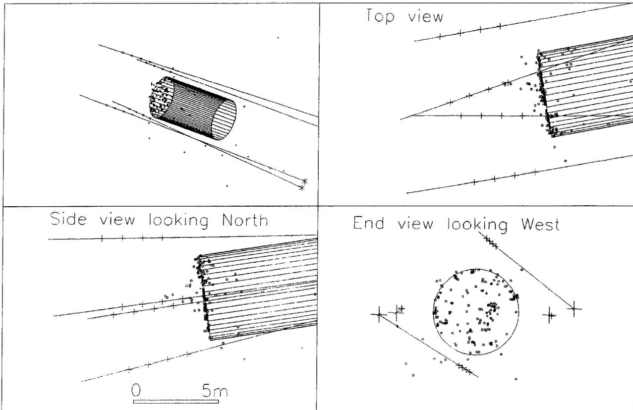
**Figure 17-3.** Acoustic Emission source locations while the tunnel boring machine was stopped overnight at 9 m from its starting position (232 events).
