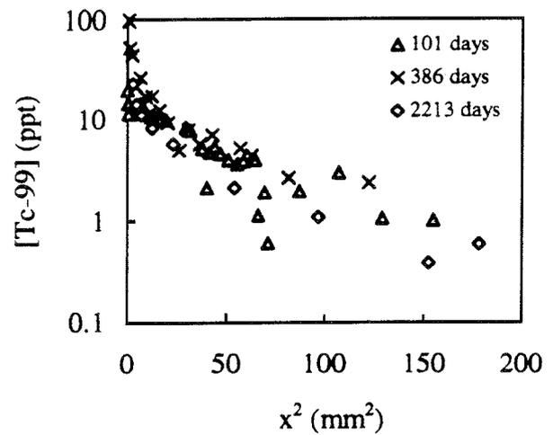
Figure 15.1-4. Diffusion profile of  $^{99}\text{Tc}$  in compacted bentonite,  $\rho_d=2100 \text{ kg/m}^3$  after different contact times.
