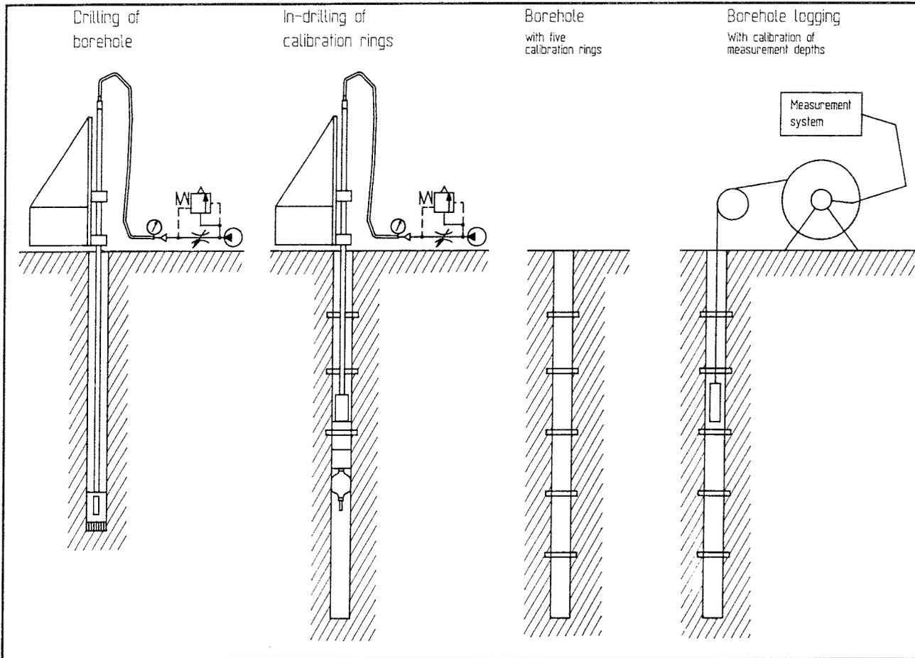
Figure 13-2. The principle of the depth calibration technique for boreholes and borehole measurements.
