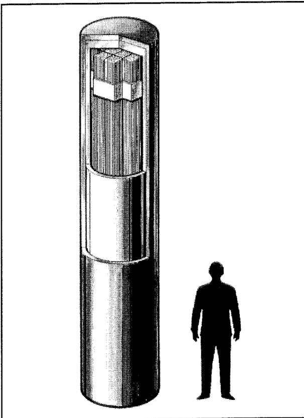
Figure 6-1. Design of canister for BWR fuel elements.
