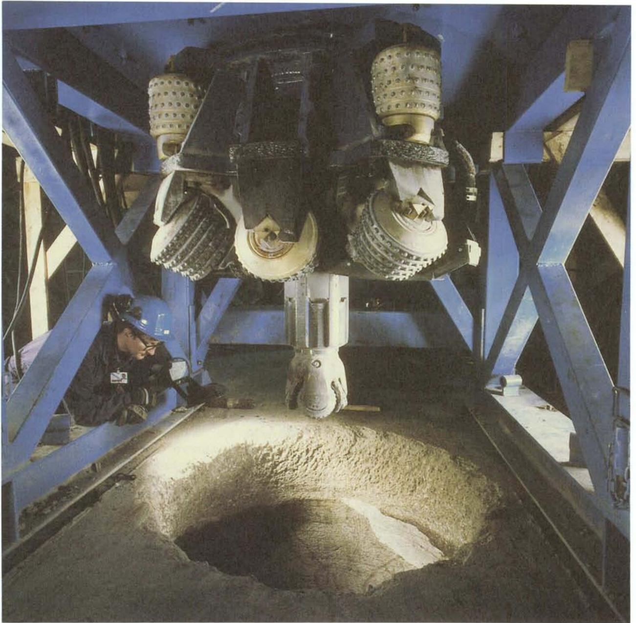
*Figure 13-6. The cutterhead.*
