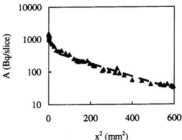
Figure 15.1-3. Diffusion profile of  $^{90}\text{Sr}$  in compacted bentonite,  $\rho_d=2100 \text{ kg/m}^3$ . The dotted line represents an apparent diffusivity of  $6.3 \cdot 10^{-12} \text{ m}^2/\text{s}$ .
