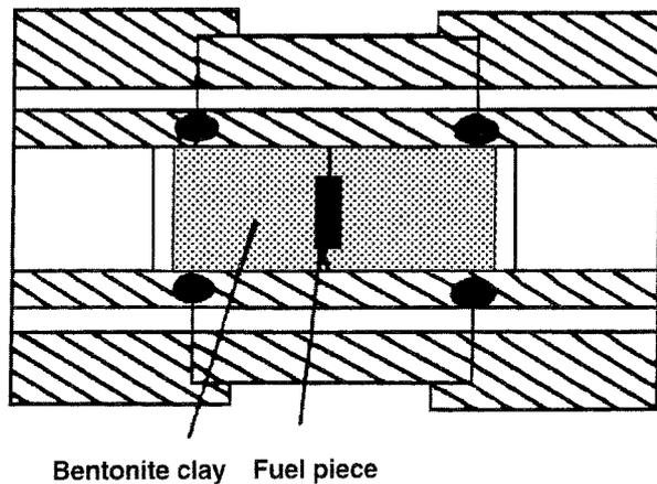
Figure 15.1-2. Schematic view of the diffusion cell.
