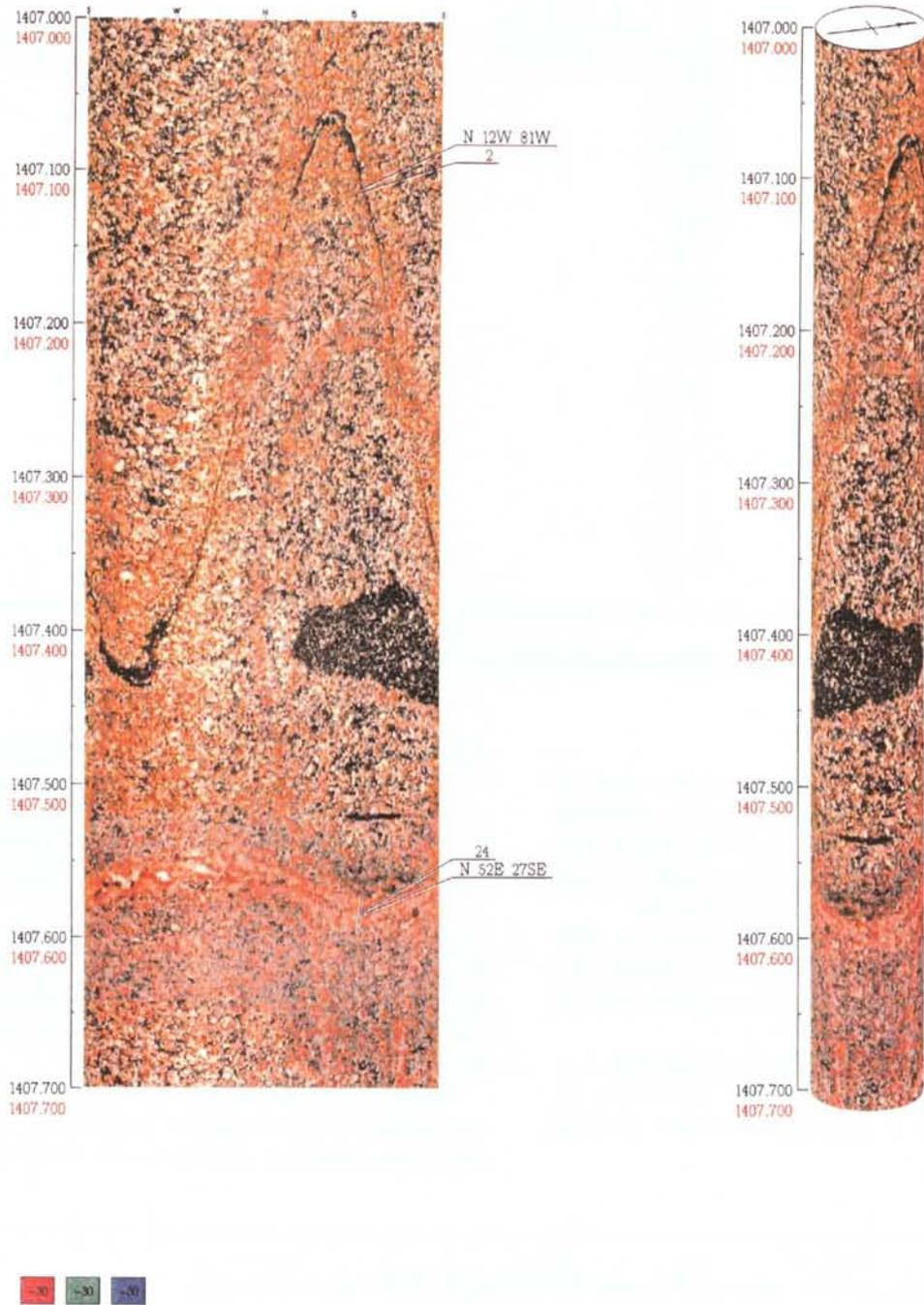
Figure 13-1. Borehole wall images from borehole KLX02, produced by BIPS-1500 borehole TV.
