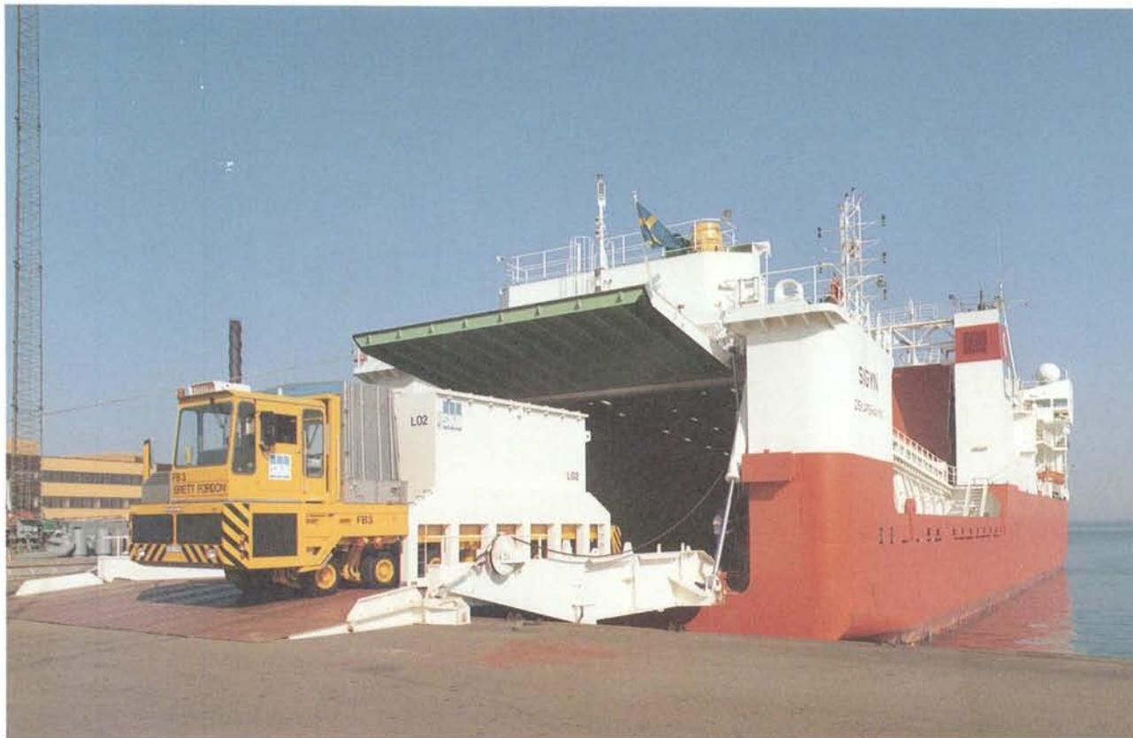
Figure 3-1. Loading of ATB-container on board M/S Sigyn.
