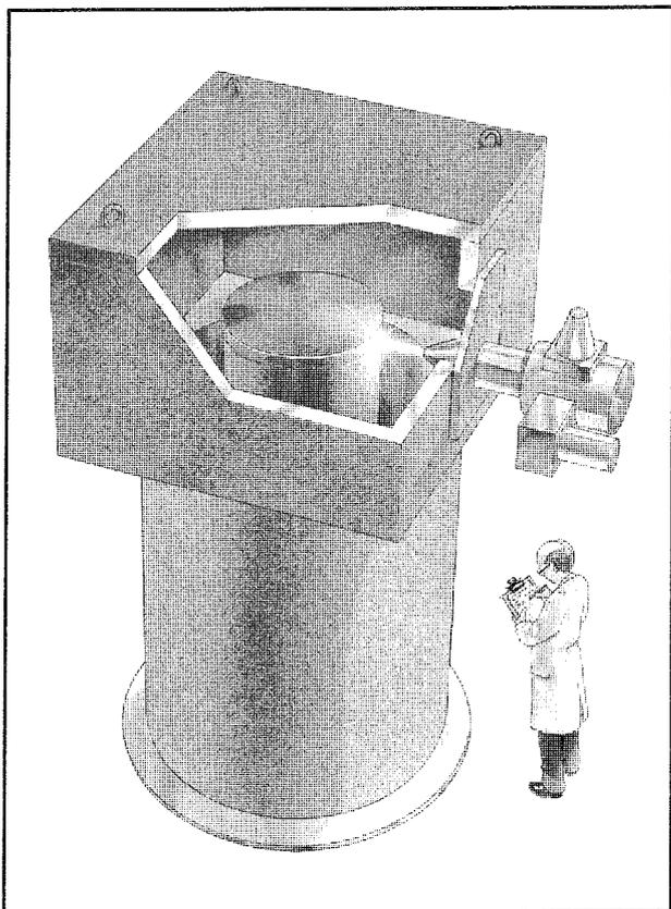
Figure 6-2. Canister lid sealing demonstration facility.
