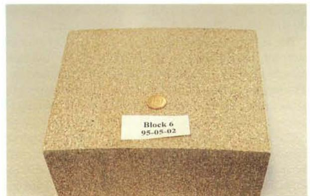
**Figure 15.2-3.** Bentonite block compacted in the Höganäs Bjuv AB brick plant for production of fireclay bricks before sintering.
