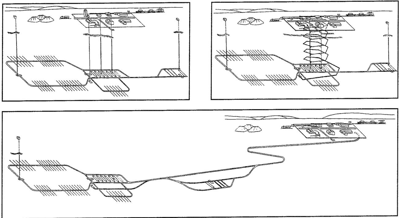
**Figure 13-4.** Schematic illustration of three alternative access systems.
