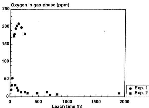
**Figure 15.1-5.** Oxygen concentration in gas phase plotted versus leach time. (1.88 g fuel, 14 cm<sup>3</sup> distilled water, 50 cm<sup>3</sup> Ar).
