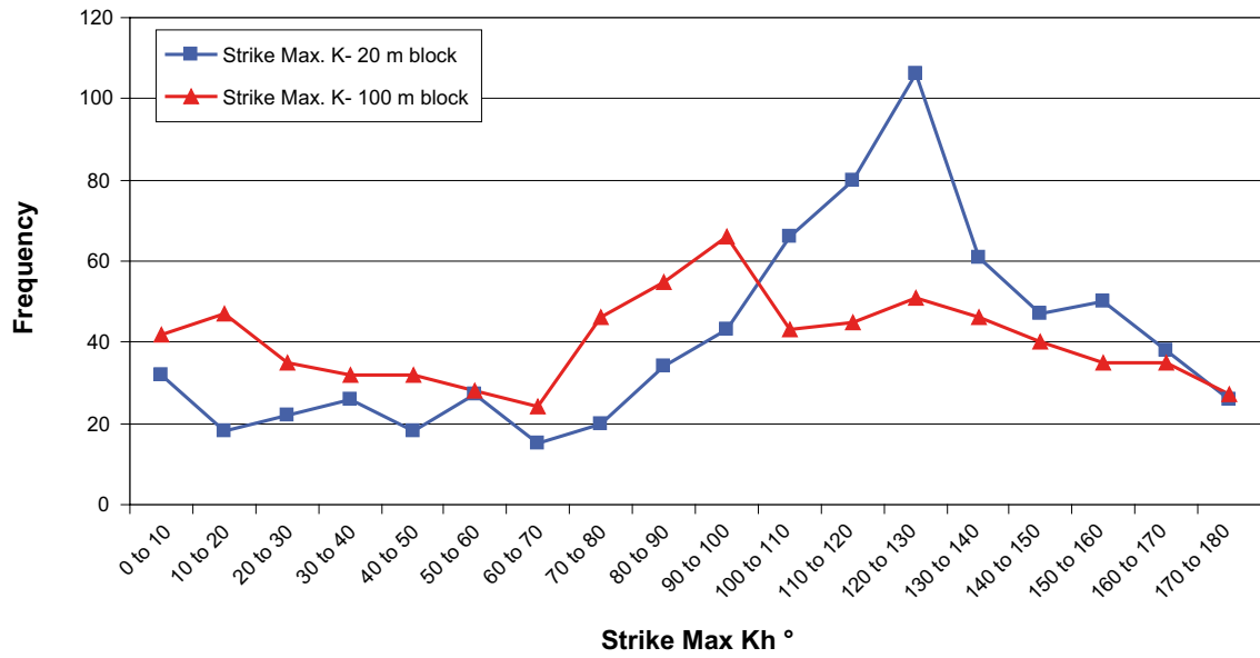
Figure 4-8. Distribution of the maximum horizontal hydraulic conductivity for the 'k r fit' case of correlated transmissivity model hydraulic data above -300 m for KLX04. Model input parameters shown in Table 3-22.
