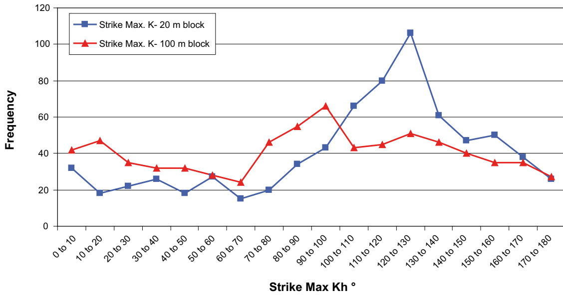
Figure 4-10. Distribution of the maximum horizontal hydraulic conductivity for the 'k r fit' case of correlated transmissivity model hydraulic data below -300 m for KLX04. Model input parameters shown in Table 3-22.
