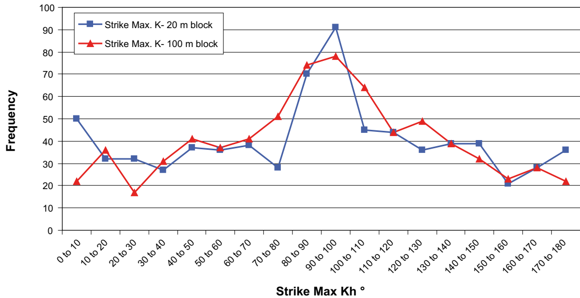
Figure 4-12. Distribution of the maximum horizontal hydraulic conductivity for the 'k r fit' case of semi-correlated transmissivity model hydraulic data above -300 m for KLX04. Model input parameters shown in Table 3-22.
