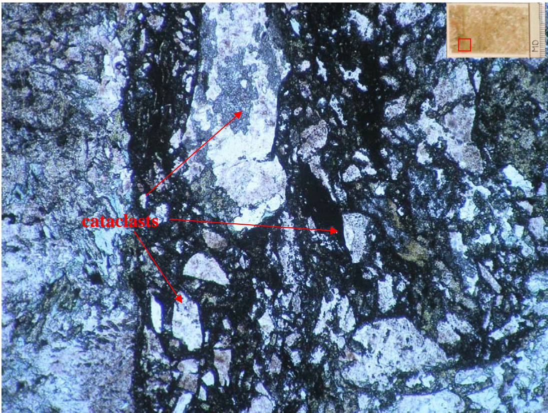
Microscope image 22: Image 21 in non-polarized light. Width of the image is 4 mm.
