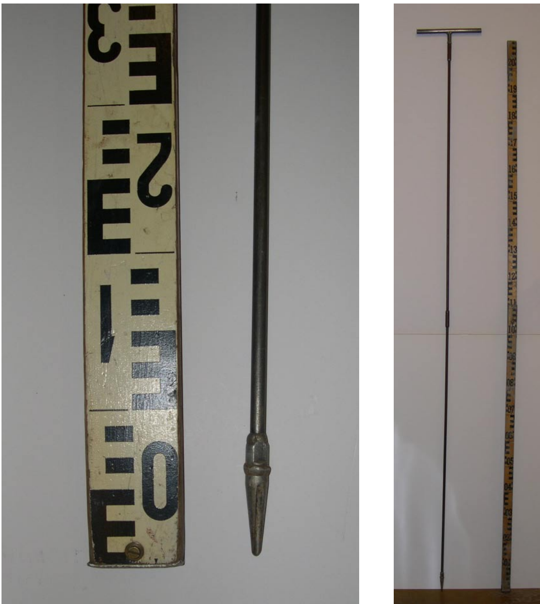
Figure 3-1. The probe with extension rods.
