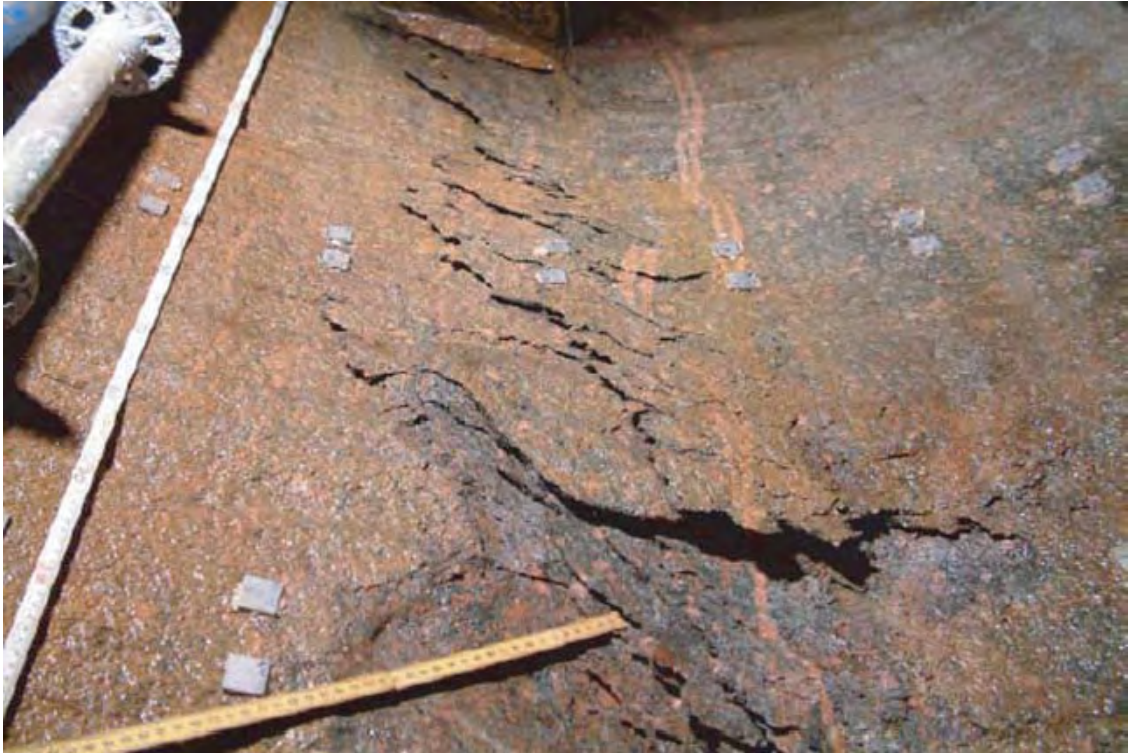
Figure 4-8. Example of spalling observed around a 1.8 m diameter borehole in the Äspö Pillar Stability Experiment (from /Martin 2005/).
