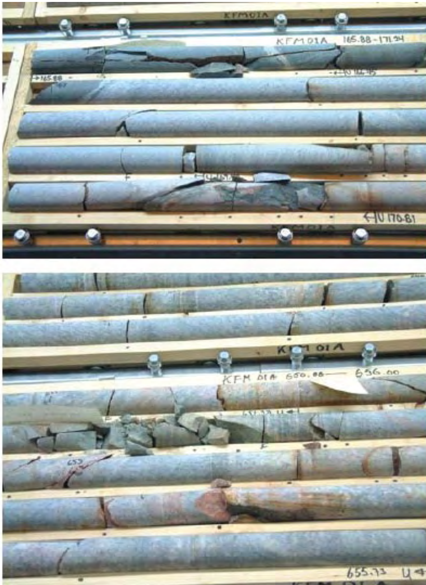
Figure 6-1. Example of fracture zones identified in borehole KFM01A. The upper zone is classified as Q=17 (most frequent value with SRF=1 ) and the corresponding value for the lower zone is Q=38 ( SRF=0.5 ) (From /Barton 2003/).
