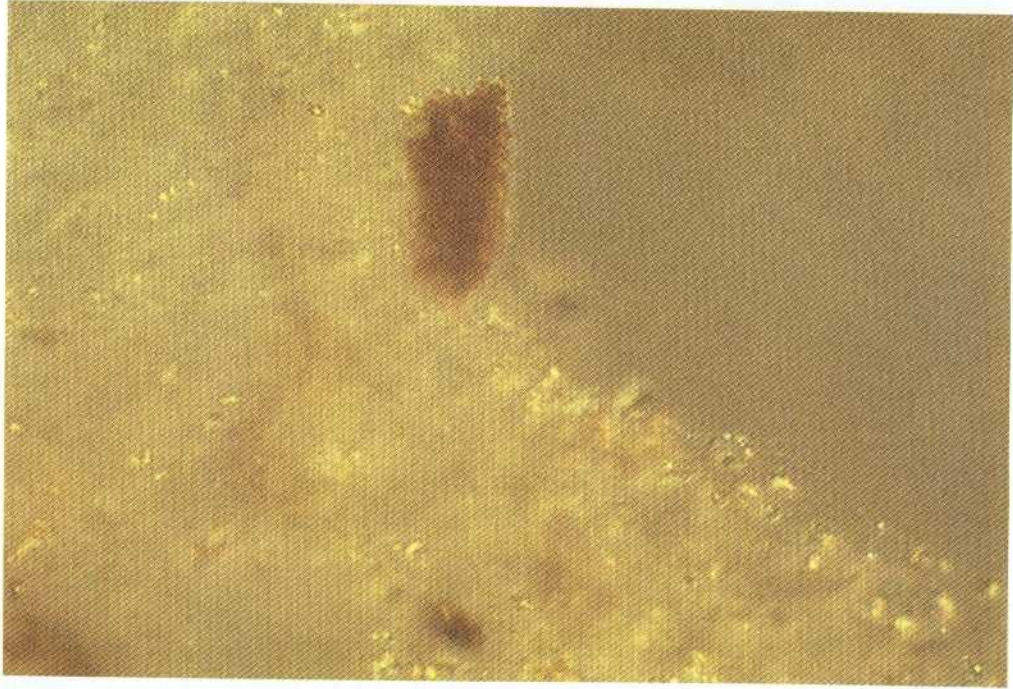
Figure 4.15 An interference light microscopy image of a wet mount of the white treads in Figure 4.11. A large amount of refractile bodies, presumably elemental sulphur can be seen, mixed with a matrix of unknown kind. Scale: 1,5 cm = 25 \mu m.
