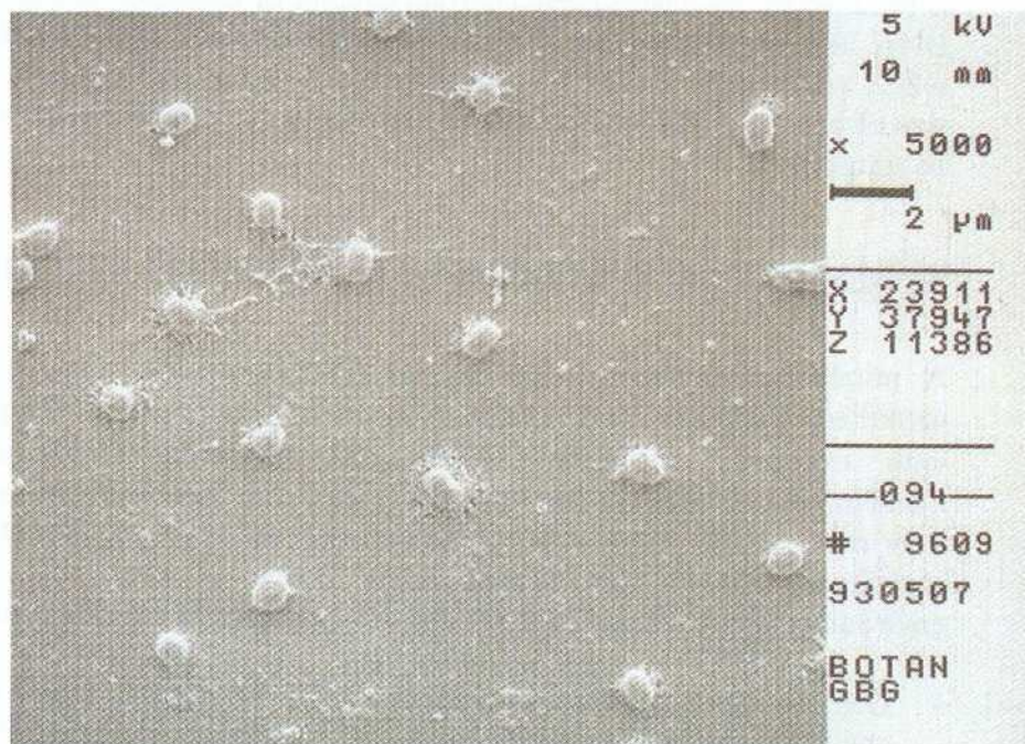
Figure 2.6 Scanning electron microscopy image of attached bacteria that grew on a surface exposed to slowly flowing groundwater from the Äspö tunnel borehole HA1327 for 70 days (179 m below ground). DNA sequencing indicates this to be new and unknown bacterial species. Bar indicates 2 \mu\text{m} .
