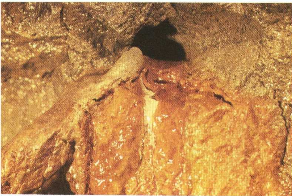
Figure 4.10 A borehole with iron precipitates that has built up since drilling of the borehole. The central white part of the motive is shown in a close up picture in Figure 4.11. The picture is from the Äspö tunnel, the B side, length 1192 m and was taken the 6 of June 1993.
