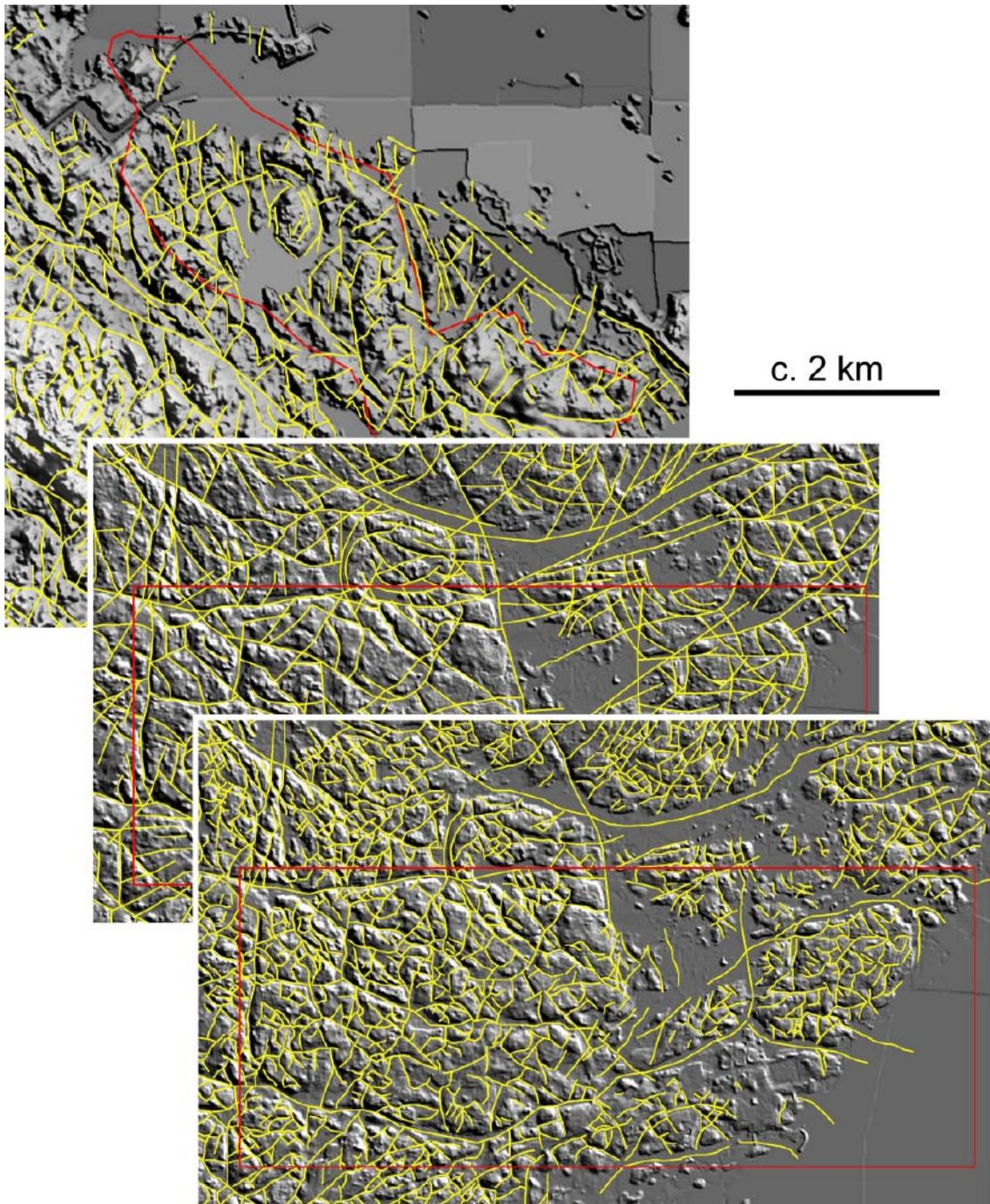
**Figure 4-15.** Forsmark topographic data and GeoVista lineament interpretation (upper), Oskarshamn topographic data and GTK (middle) and GeoVista (lower) lineament interpretations. The Forsmark candidate area and the Laxemar local scale model area are outlined in red.
