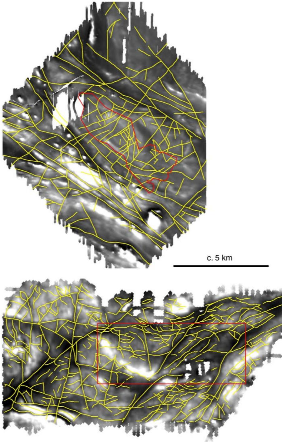
*Figure 4-16. Forsmark airborne magnetic data and GeoVista lineament interpretation (upper) and Oskarshamn airborne magnetic data and GeoVista lineament interpretation (lower). The Forsmark candidate area and the Laxemar local scale model area are outlined in red.*
