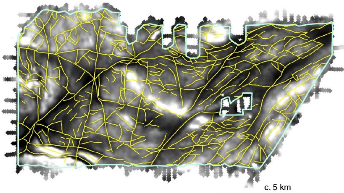
**Figure 4-4.** The primary (GeoVista) interpretation of magnetic lineaments (yellow) superimposed on a grey scale presentation (positive anomalies light, negative anomalies dark) of the magnetic anomaly. The area of interpretation is outlined in light blue.
