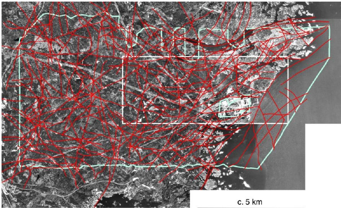
**Figure 4-11.** The alternative (GTK) interpretation of linked lineaments longer or equal to 1,000 m (red) superimposed on a mosaic of grey scale orthophotos. The area of combined interpretation is outlined in light blue and the Laxemar local scale model area in white.
