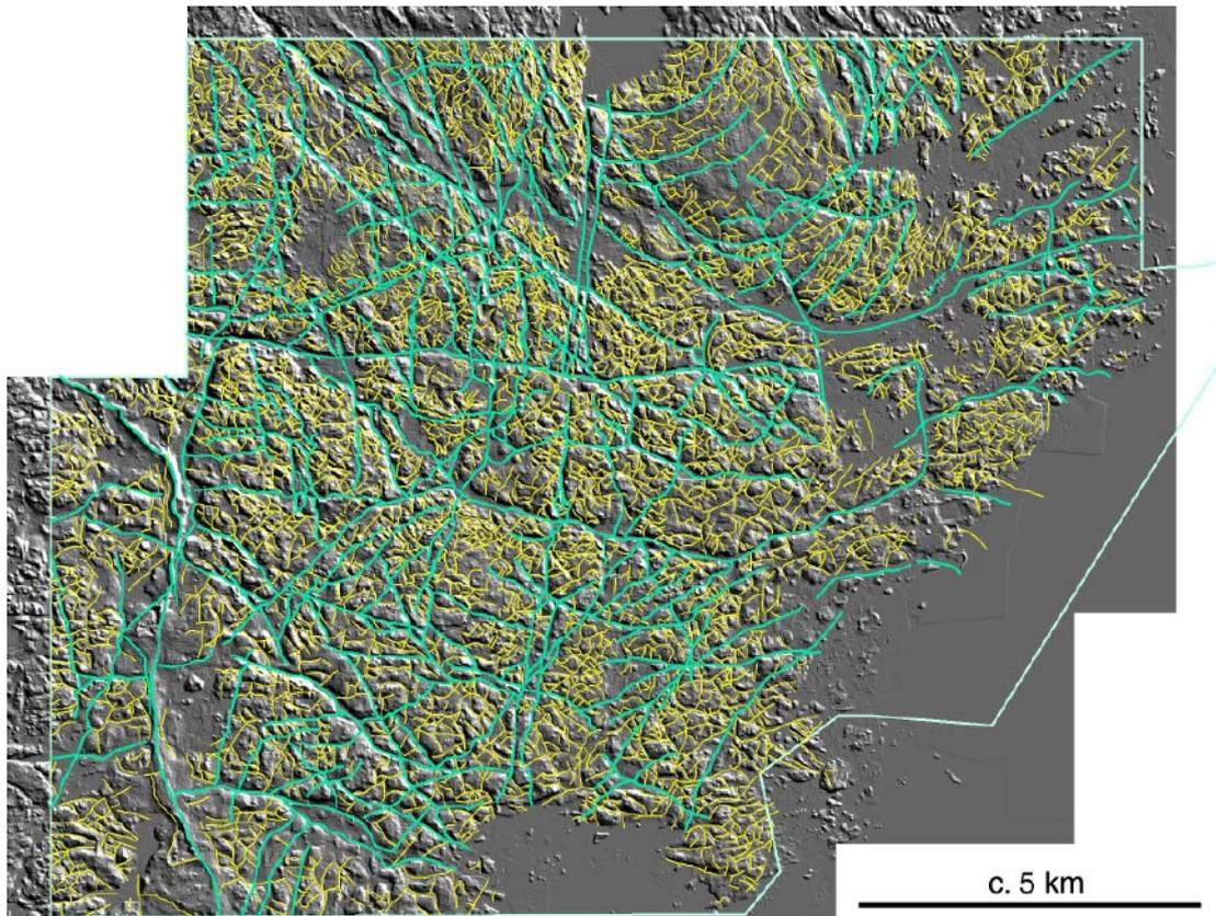
**Figure 4-3.** Topographic GeoVista lineaments superimposed on a grey scale presentation of the digital terrain model. Lineaments classified as “major” or “local major” in blue, “local minor” lineaments in yellow. The area of topographic interpretation is outlined in light blue.
