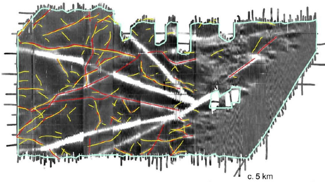
**Figure 4-9.** VLF lineaments superimposed on a grey scale presentation (positive anomalies light, negative anomalies dark) of the VLF total field orthogonal station data. The primary (GeoVista) interpretation is shown in yellow and the alternative (GTK) interpretation in red. The area of interpretation is outlined in light blue.
