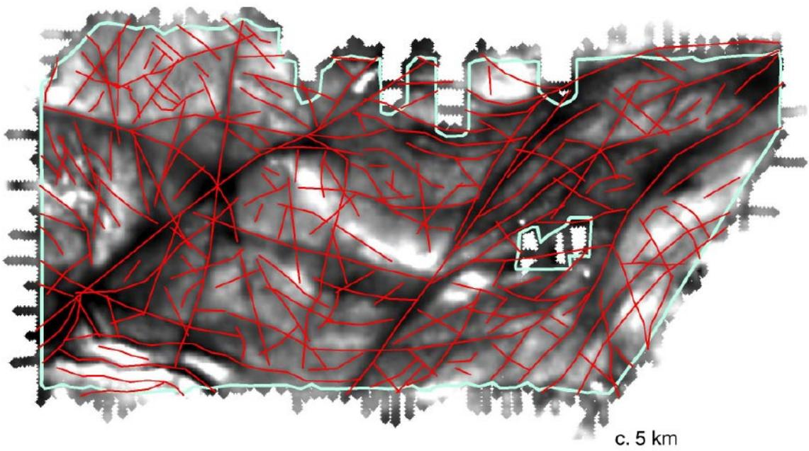
**Figure 4-5.** The alternative (GTK) interpretation of magnetic lineaments (red) superimposed on a grey scale presentation (positive anomalies light, negative anomalies dark) of the magnetic anomaly. The area of interpretation is outlined in light blue.
