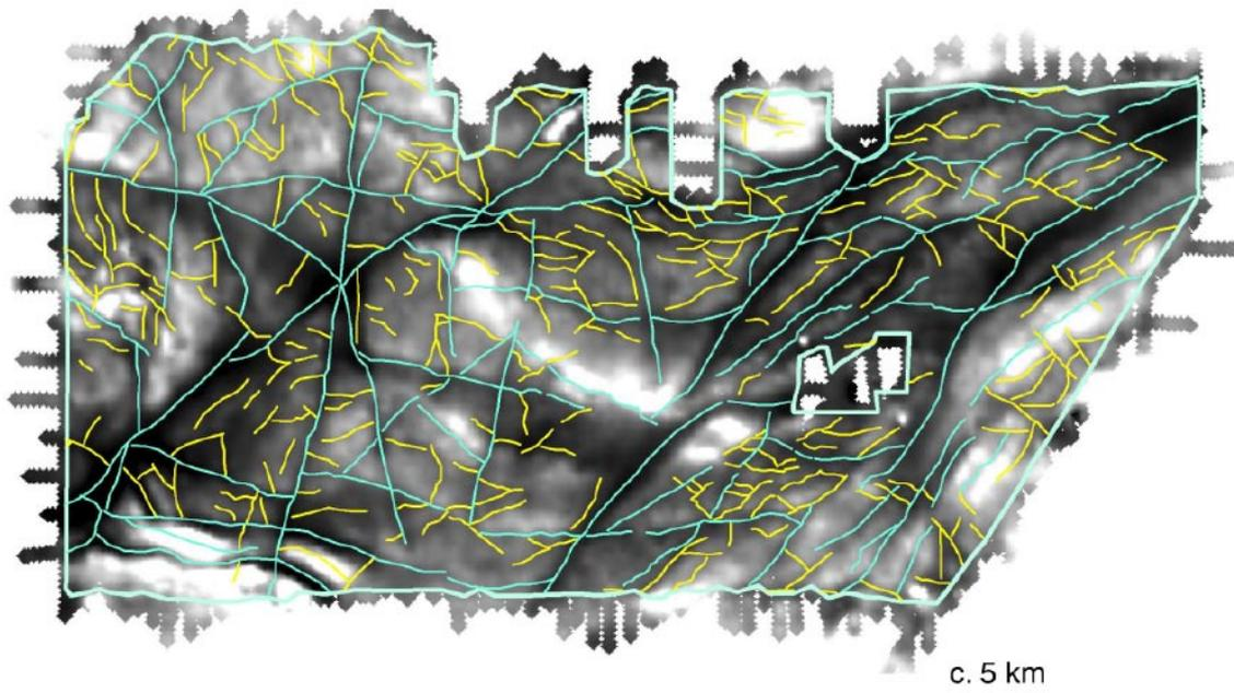
**Figure 4-6.** Magnetic GeoVista lineaments superimposed on a grey scale presentation (positive anomalies light, negative anomalies dark) of the magnetic anomaly. Lineaments classified as "local major" in blue, "local minor" lineaments in yellow. The area of interpretation is outlined in light blue.
