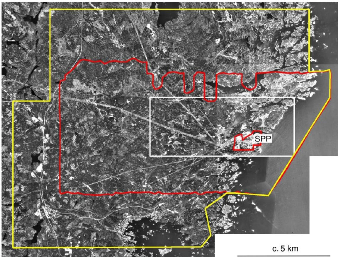
**Figure 2-1.** The areas of interpretation. The common area for topographic interpretation is outlined in yellow and the helicopter survey area in red. The latter area is also the area for integrated geophysical and topographic interpretation. The white rectangle shows the Laxemar local scale model area. SPP=Simpevarp nuclear power plant.
