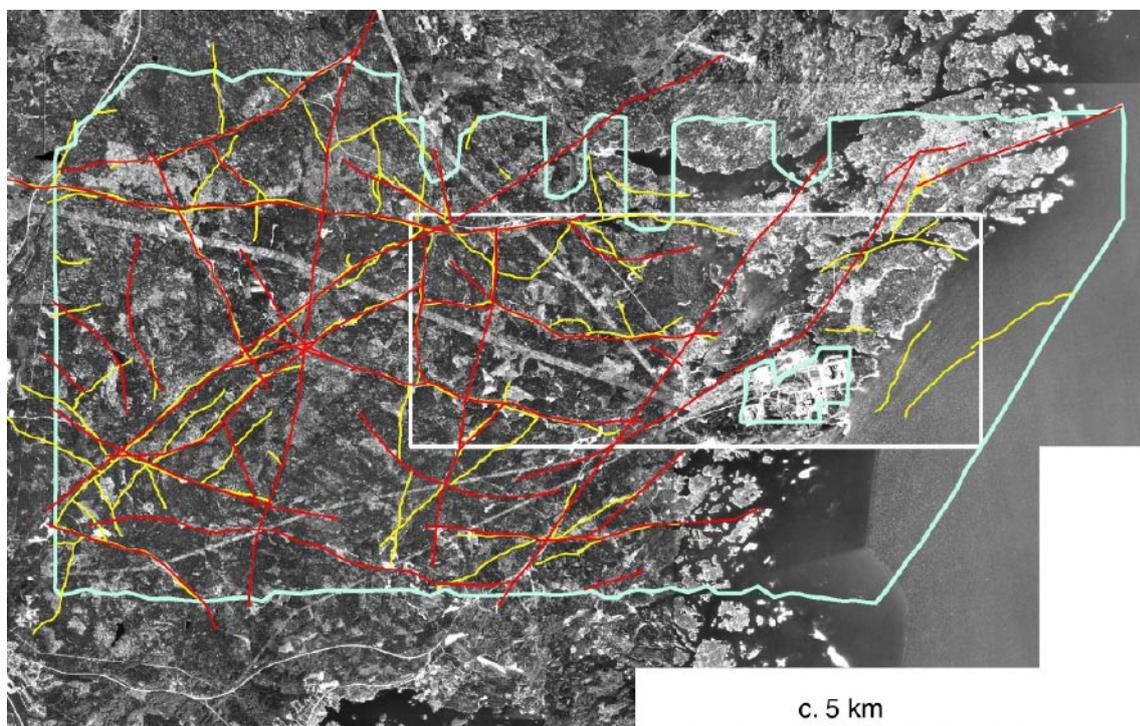
**Figure 4-14.** Linked lineaments, weight > 3.5, superimposed on a mosaic of grey scale ortho-photos. The primary (GeoVista) interpretation is shown in yellow and the alternative (GTK) interpretation in red. The area of combined interpretation is outlined in light blue and the Laxemar local scale model area in white.
