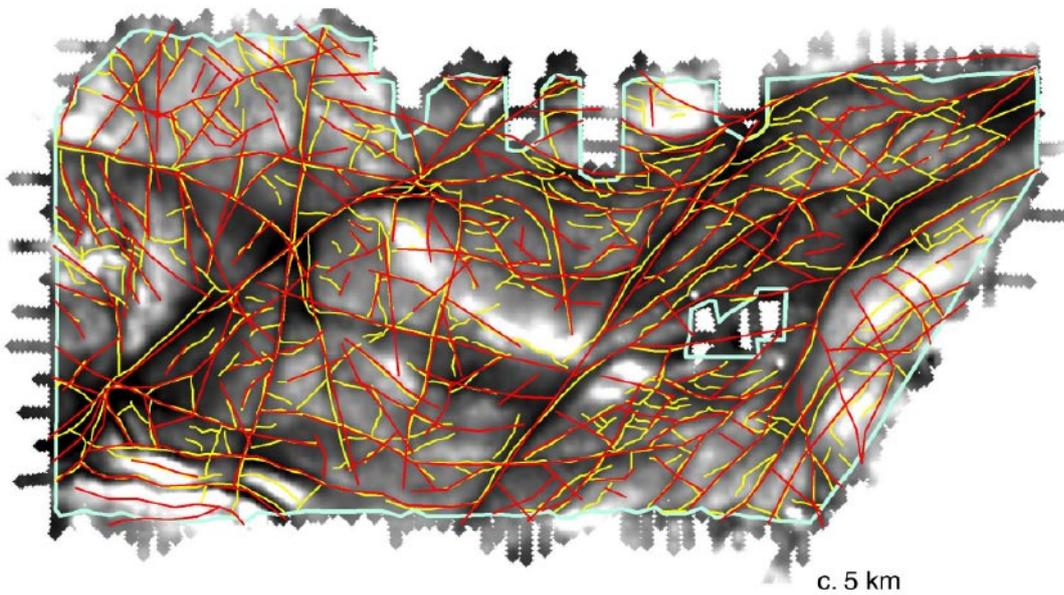
**Figure 4-7.** Magnetic lineaments superimposed on a grey scale presentation (positive anomalies light, negative anomalies dark) of the magnetic anomaly. The primary (GeoVista) interpretation is shown in yellow and the alternative (GTK) interpretation in red. The area of interpretation is outlined in light blue.
