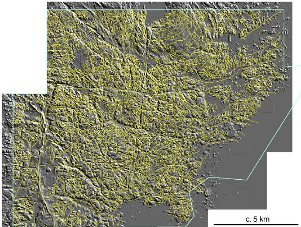
**Figure 4-1.** The primary (GeoVista) interpretation of topographic lineaments (yellow) superimposed on a shaded (from NE) grey scale presentation of the digital terrain model. The area of topographic interpretation is outlined in light blue.
