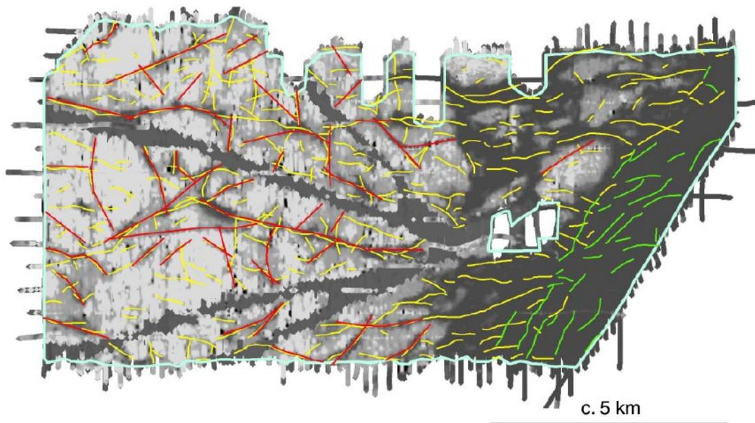
**Figure 4-8.** Electromagnetic (dipole source) lineaments superimposed on a grey scale presentation (high resistivity areas light, low resistivity areas dark) of the apparent resistivity (800 Hz) map. The primary (GeoVista) interpretation is shown in yellow and the alternative (GTK) interpretation in red. GeoVista interpretation in the sea area based on inverted helicopter EM data (sea-floor depressions) is shown in green. The area of interpretation is outlined in light blue.
