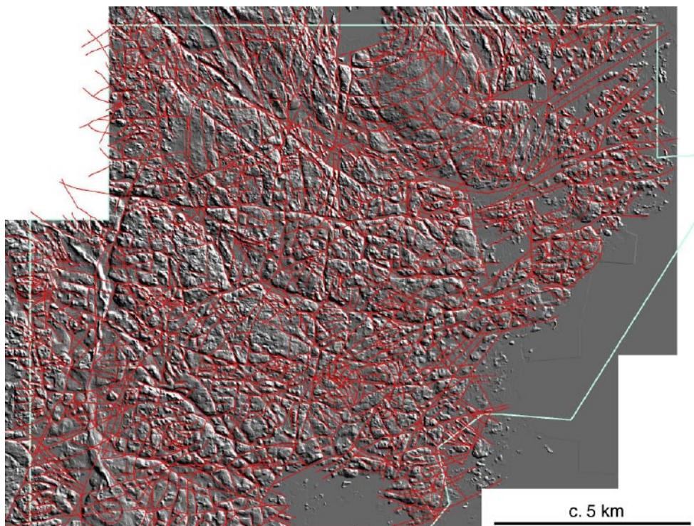
**Figure 4-2.** The alternative (GTK) interpretation of topographic lineaments (red) intersecting the area of topographic interpretation superimposed on a shaded (from NE) grey scale presentation of the digital terrain model. The area of topographic interpretation is outlined in light blue.
