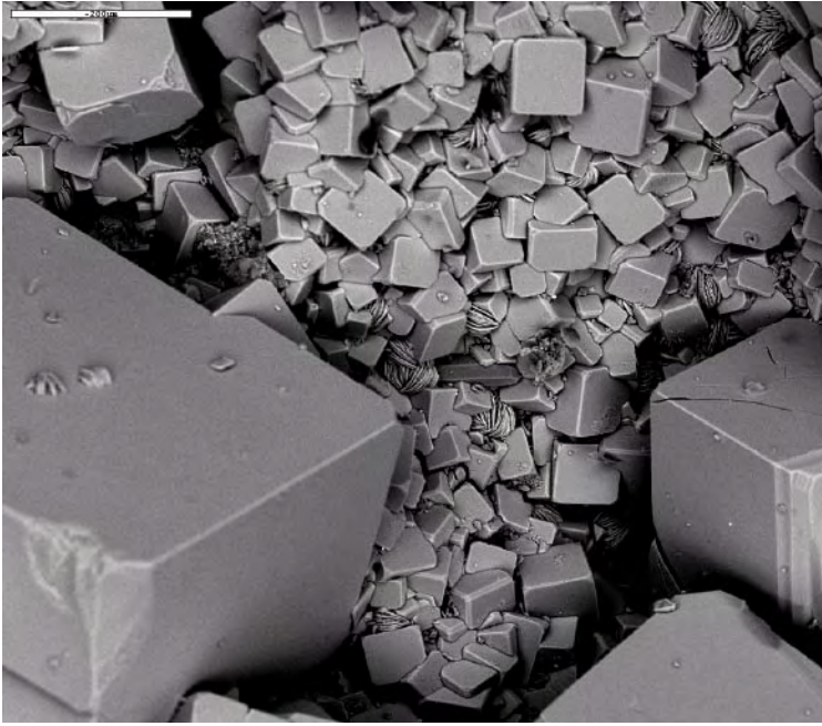
Back-scattered SEM-image of mostly cubic fluorite crystals of variable size. Minor amounts of darker quartz crystals and platy Fe-rich chlorite crystals. Scale bar is 200 \mu\text{m} .
