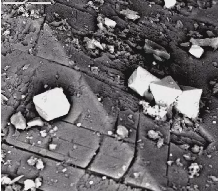
Back-scattered SEM-image of bright pyrite crystals on the surface of a calcite crystal. Scale bar is 20 \mu\text{m} .
