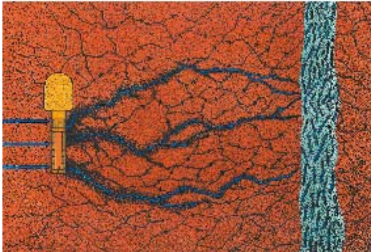
Figure 10-2. Schematic representation of flow and transport in the “immediate far-field” conceptualised to be the first 10–100 m between any given canister hole and the nearest large scale deformation zone.
