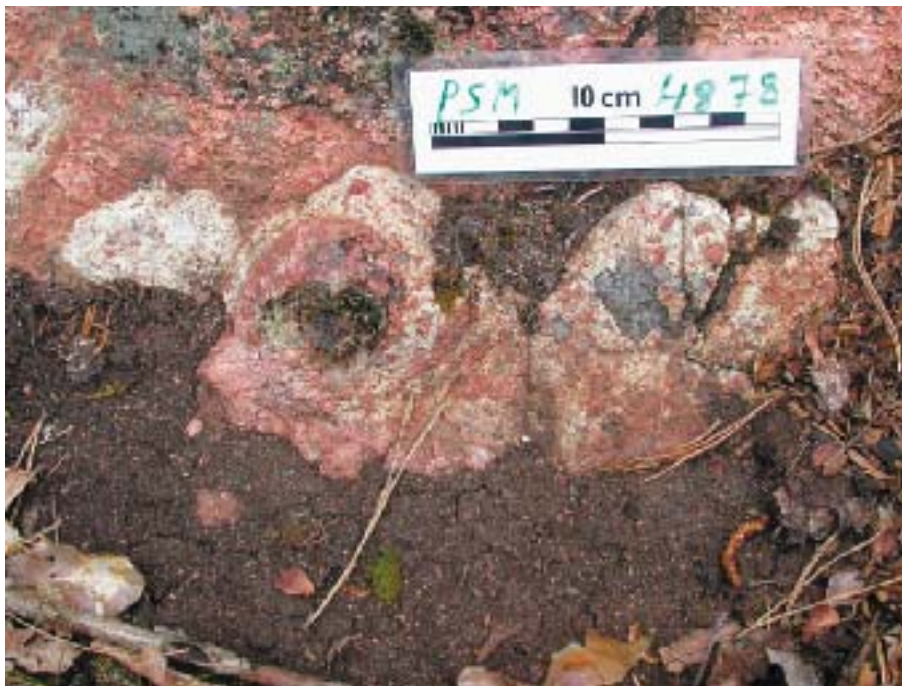
Figure 5-29. Brittle deformation and red staining in Ävrö granite close to the deformation zone ZSMNW929A (see section Figure 5-72) in the northern part of the Laxemar subarea. Note the red staining (oxidation).
