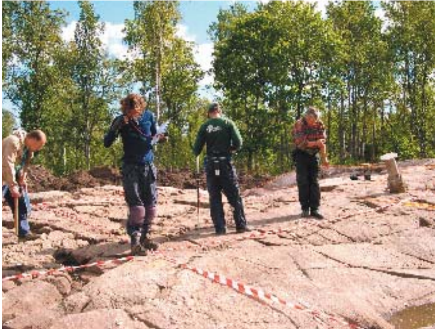
Figure 5-27. Detailed fracture mapping on the cleaned outcrop ASM000209 in southern Laxemar. Drill site for cored borehole KLX05, cf. Figure 5-26.
