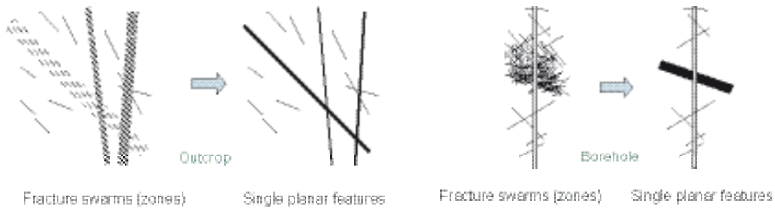
Figure 8-10. Potentially flowing stochastic deformation zones consisting of fracture swarms (clusters) are simulated as single planar features and are considered homogeneous with regards to their hydraulic properties /Follin et al. 2006/.
