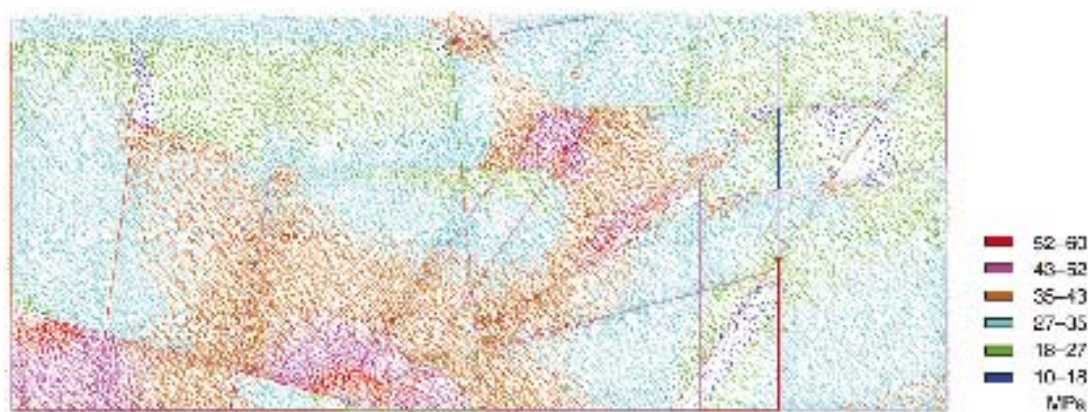
Figure 6-17. Modelled principal stress trajectories in a horizontal plane at 450 m depth. The colours indicate the magnitude of the major principal stress. It may be noted that the stresses differs quite substantially within the local area of this 3DEC model. Note that the colour code scales are not the same in the horizontal and vertical sections (see legends).
