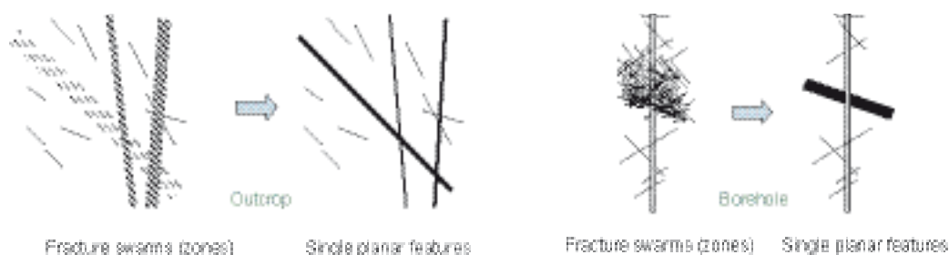
Figure A8-1. Potentially flowing stochastic deformation zones consisting of fracture swarms (clusters) are simulated as single planar features and are considered homogeneous with regards to their hydraulic properties /Follin et al. 2006/.
